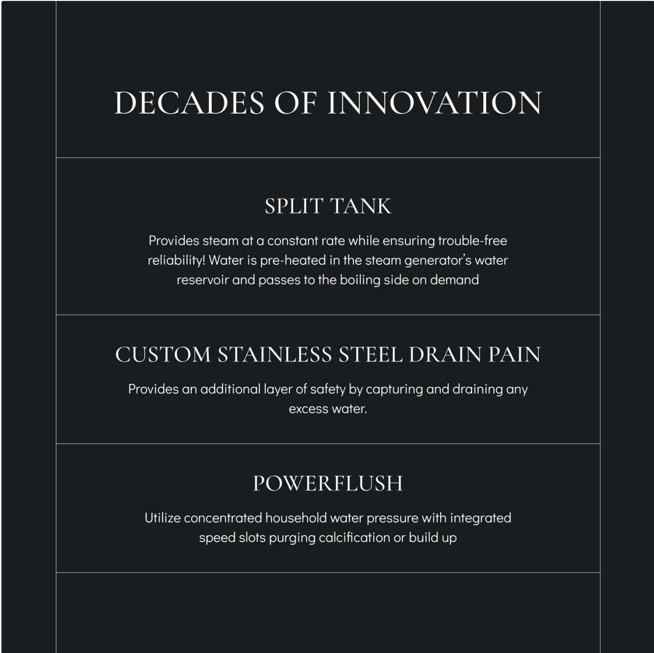
Figure 5: Innovations in ThermaSol steam generator design.
