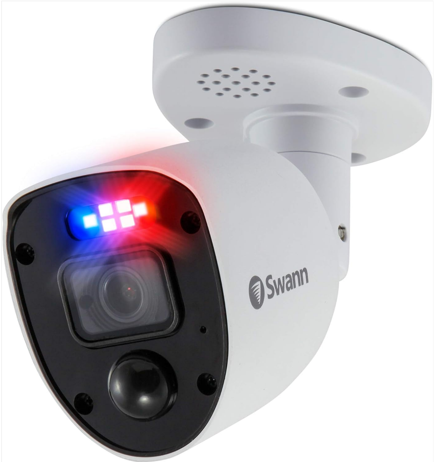
Image: Front view of the SwannForce camera, showcasing its active red and blue flashing lights and sensor spotlight.
