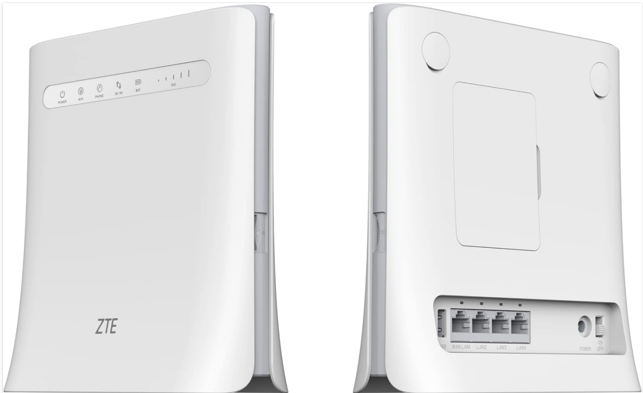
Figure 3.2: Rear Panel Ports of ZTE MF286C Router. This image provides a clear view of the router's rear panel, highlighting the WAN/LAN port, three additional LAN ports, the power input, and the power on/off switch. The SIM card slot is located under a cover on the back.
