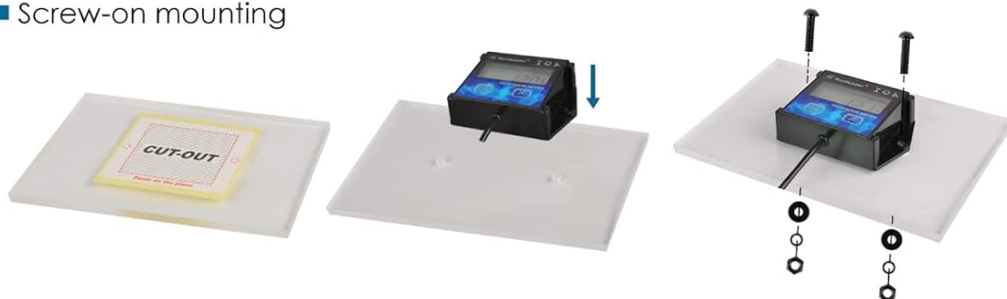
Figure 5: Illustration of stick-on, snap-in, and screw-on mounting methods.
