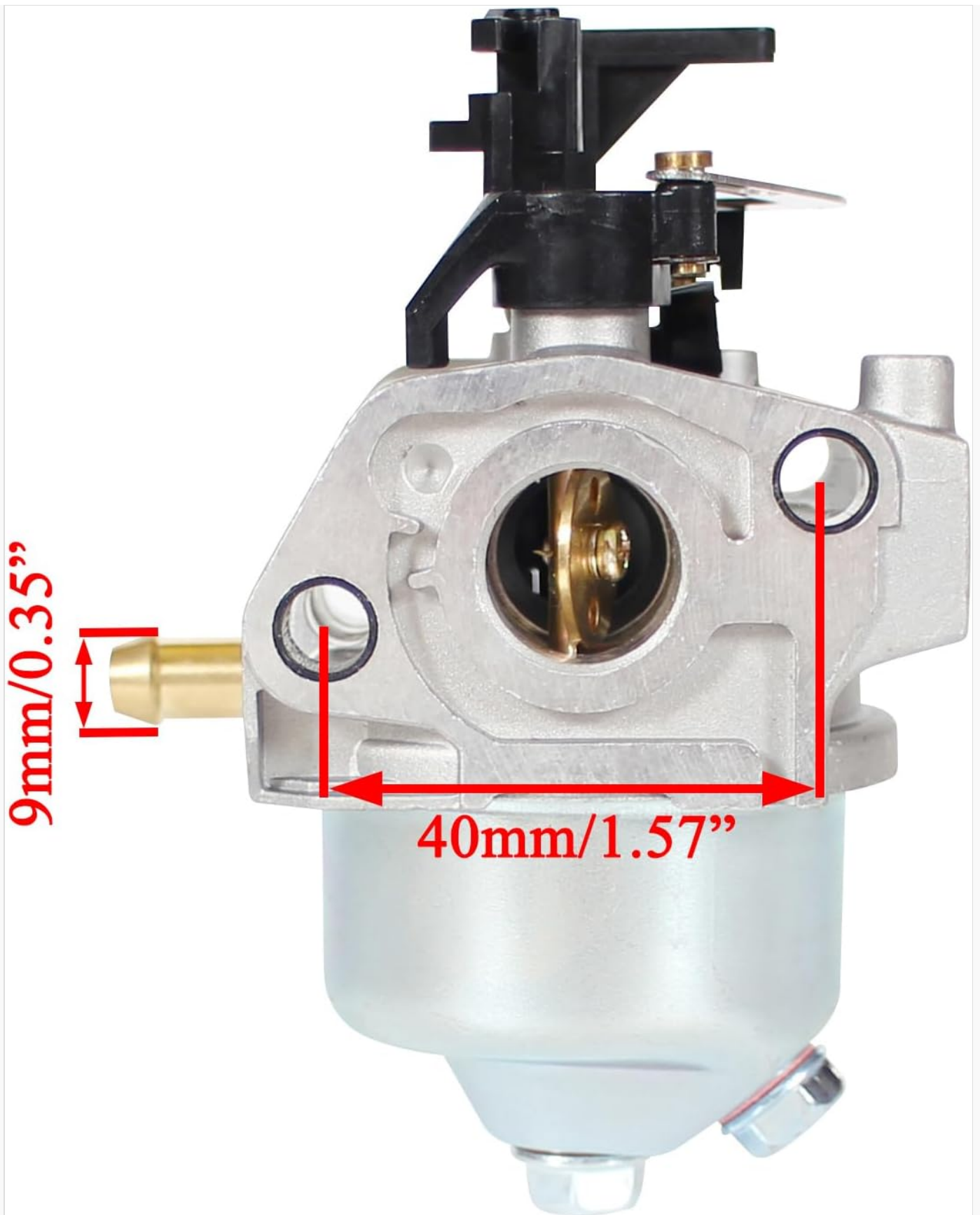
Image 4.2: Side view of the carburetor with key dimensions (e.g., 40mm / 1.57" mounting hole spacing, 9mm / 0.35" fuel inlet diameter).
