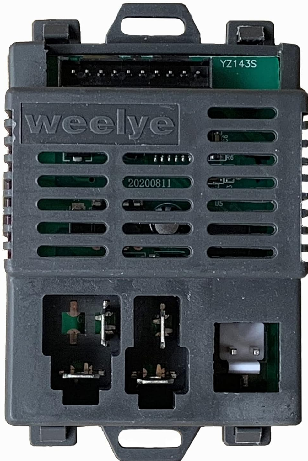
Image 1: Top view of the Weelye RX25 6V Control Box. Note the "weelye" branding and connector layout.
