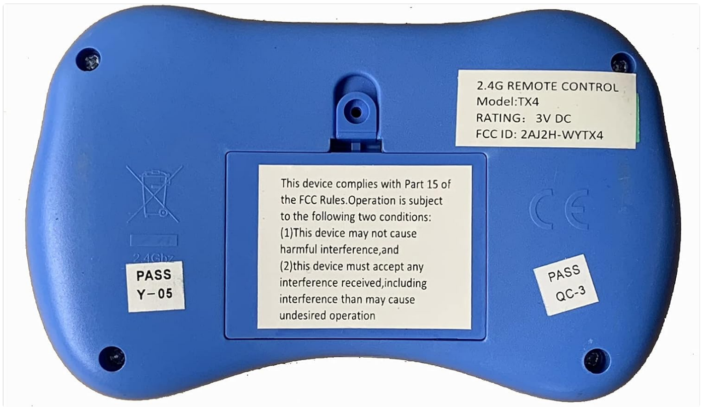
Image: Rear view of the blue weelye TX4 remote control, displaying the battery compartment, FCC ID (2AJ2H-WYTX4), and compliance information.
