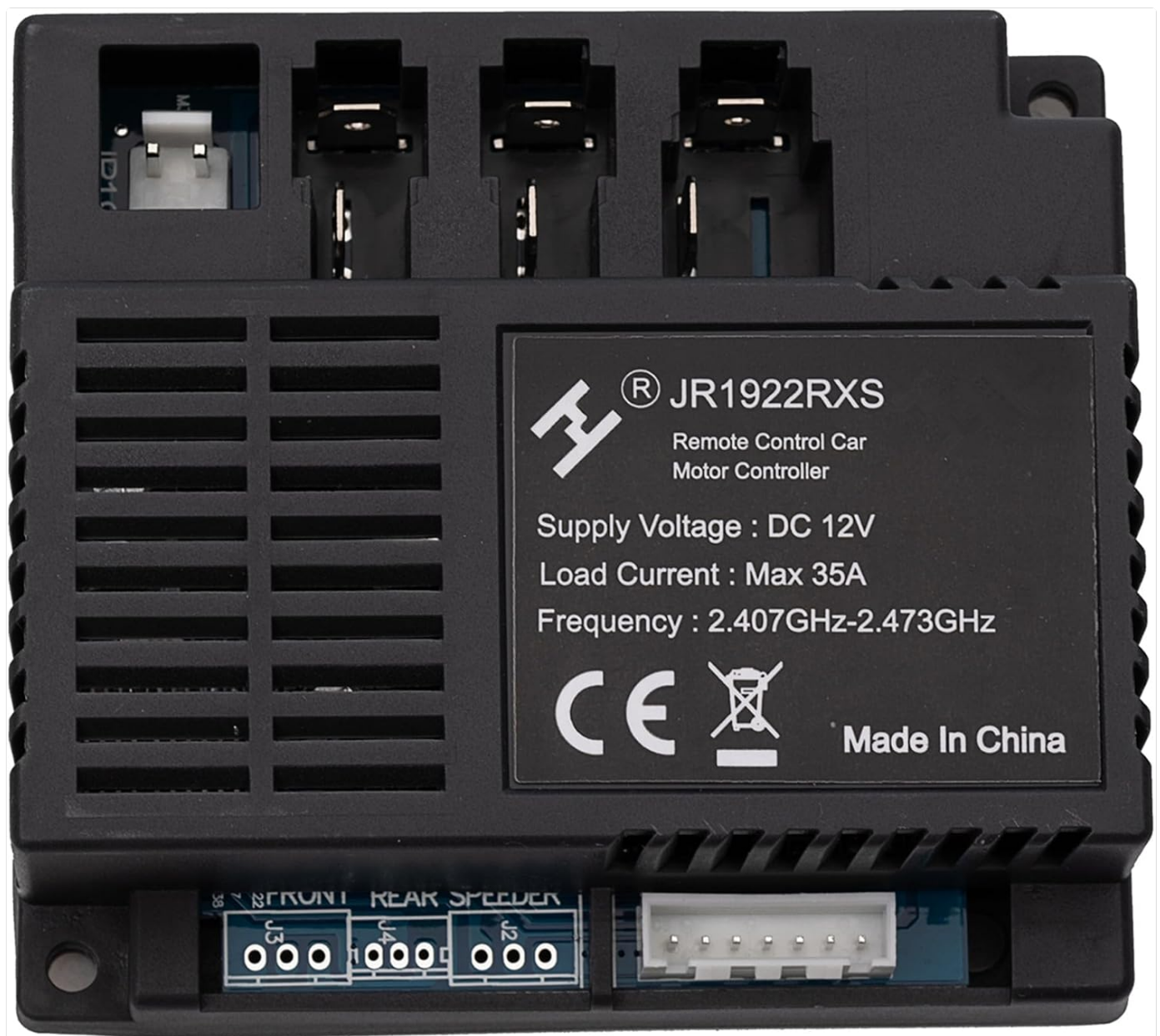
Image 1.1: weelye JR1922RXS Receiver Control Box. This image shows the top view of the black receiver unit with connection ports and product labeling.
