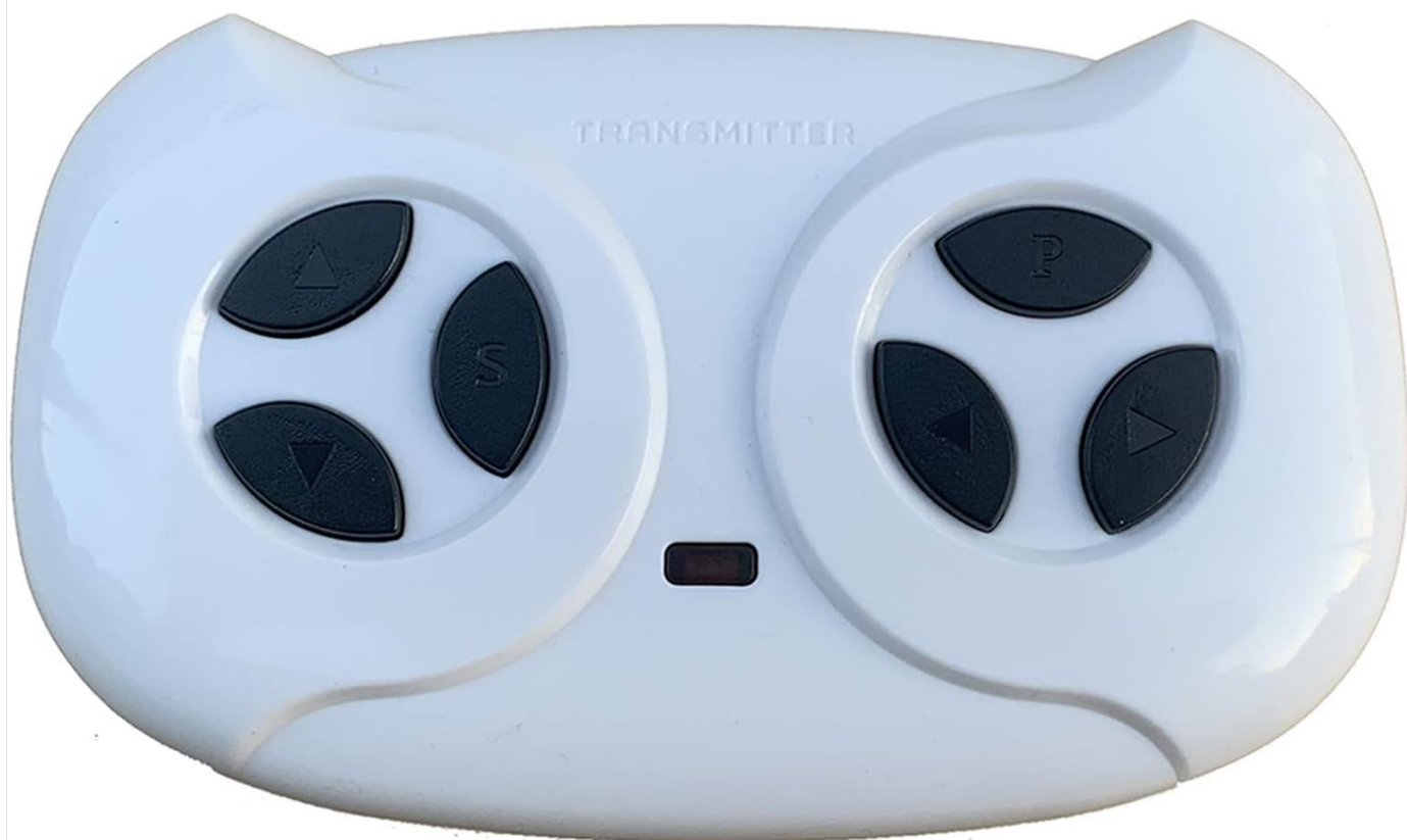
Image 1.2: weelye 2.4G Bluetooth Remote Control. This image displays the white remote control with directional, speed, and brake buttons.
