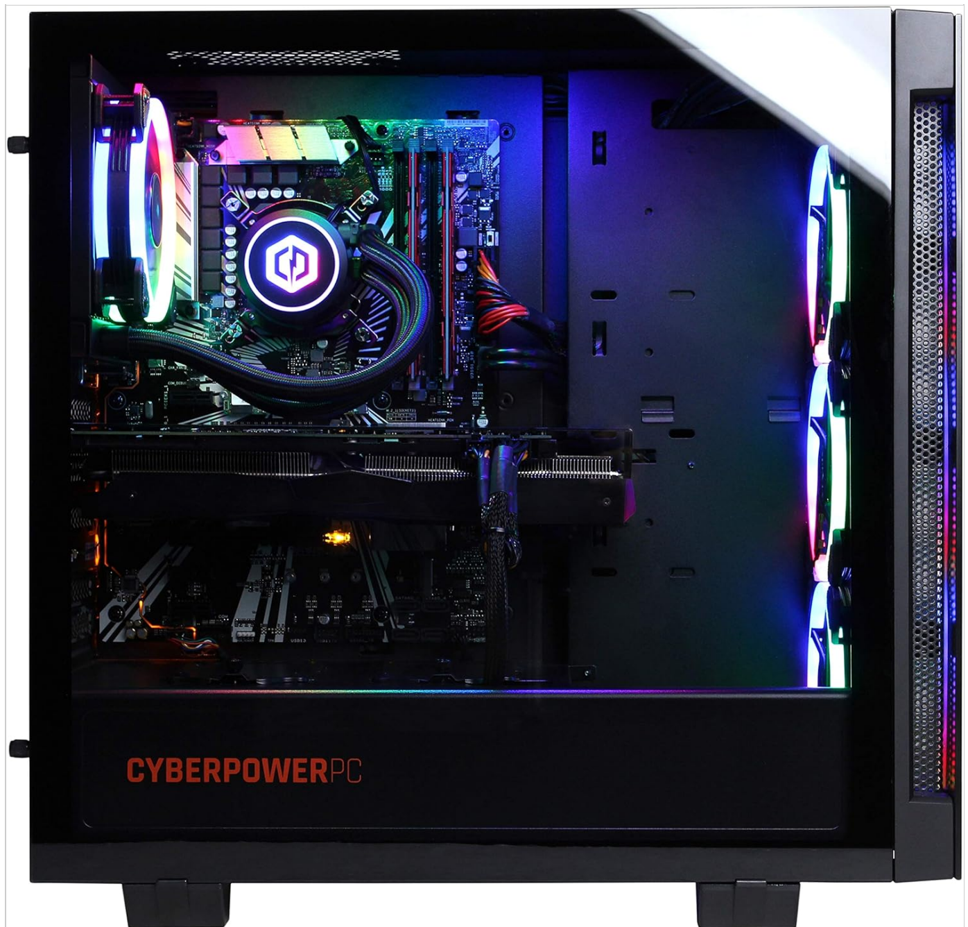
Figure 3: Internal view of the PC tower showcasing the liquid-cooled CPU, RAM, and GPU with custom RGB lighting.
