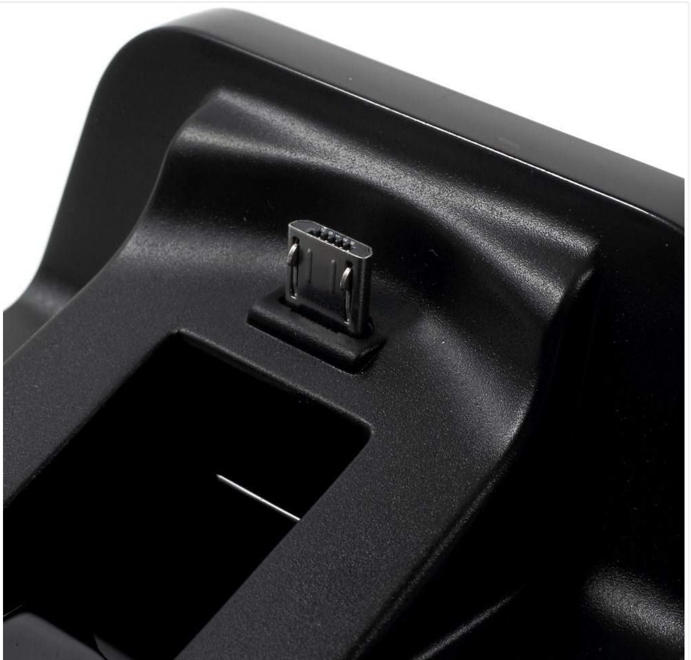
Figure 3: Close-up view of one of the micro USB charging ports on the dock, where the controller connects.
