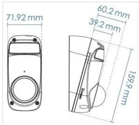
Image: Dimensional diagram of the VIVOTEK CC9381-HV camera.
