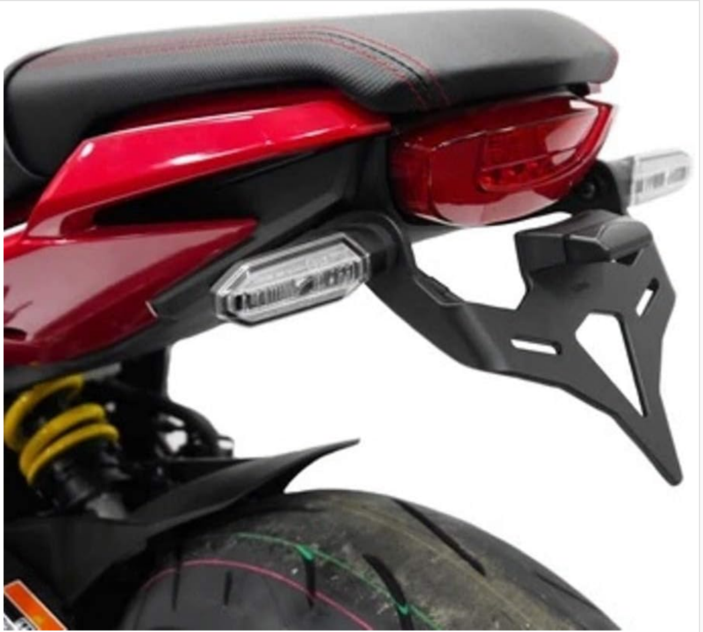
Figure 3: Rear-side view of the installed Tail Tidy, showing the license plate mounting area and the integration of the standard signal lights.
