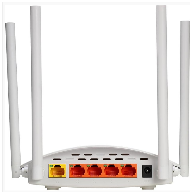
Figure 2.2.2: Rear view of the Totolink N600R router, highlighting the WAN port (yellow), four LAN ports (orange), and the DC power input.
