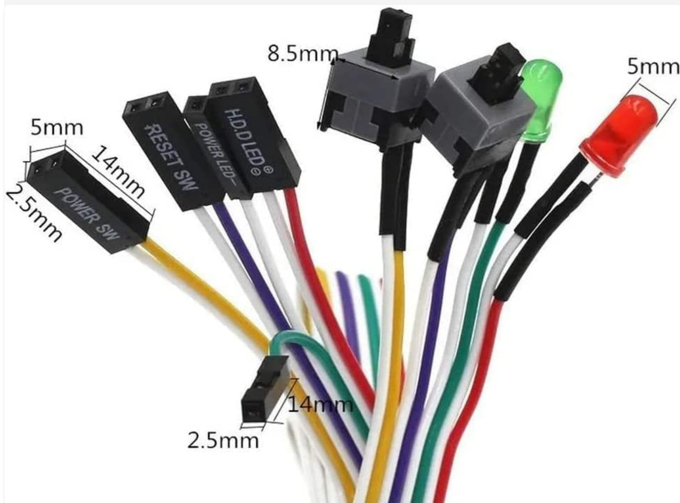
Image: The individual connectors of the DTech PC Front Panel Cable Kit, illustrating their approximate dimensions for reference during installation.
