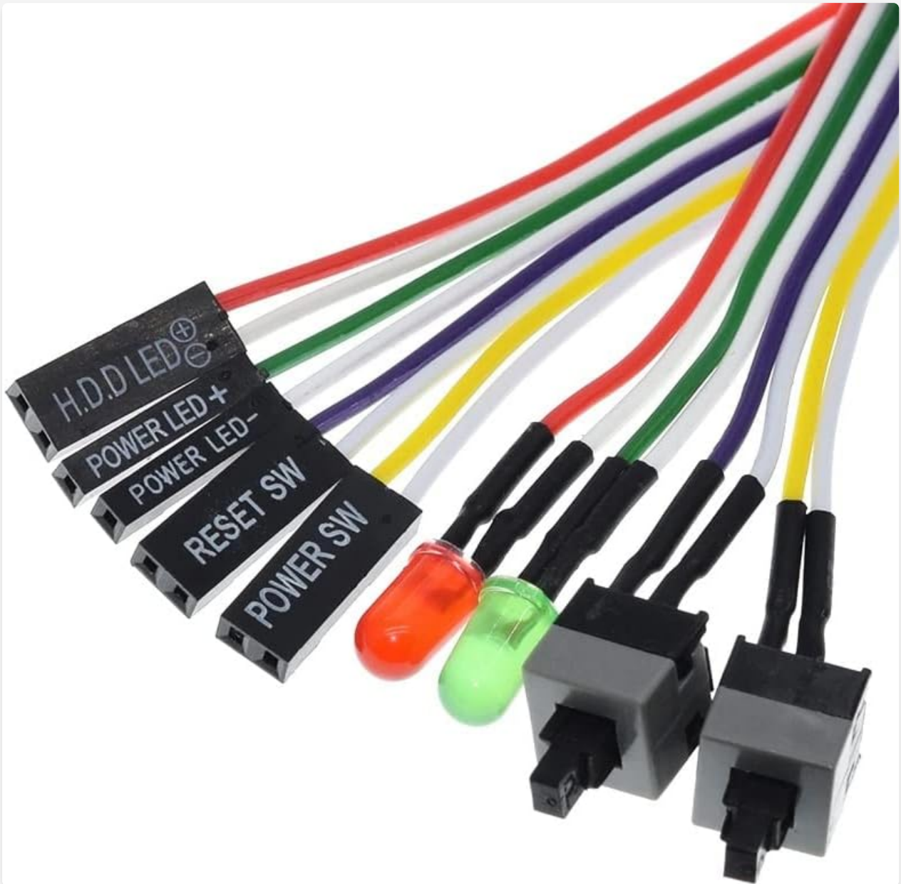
Image: A close-up view of the individual connectors (POWER SW, RESET SW, POWER LED, H.D.D LED) with their respective labels, showing the distinct wires and their polarity markings for the LEDs.
