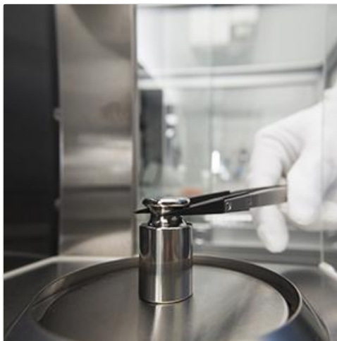
Figure 4: A close-up view of the uxcell 20g F1 Precision Calibration Weight, showing its smooth, polished stainless steel surface.
