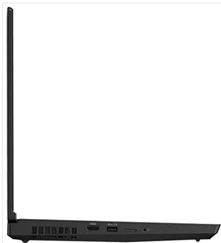
Figure 4: Left side of the workstation, displaying ports such as USB and audio jack.
