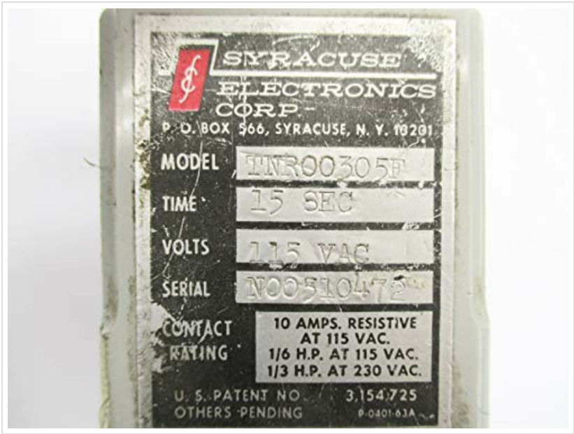
Figure 3: Product label of the TNR00305F, detailing electrical specifications.
