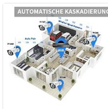
Figure 3: Automatic Cascading. This diagram illustrates how cameras can relay signals to the NVR, improving coverage in larger areas.
