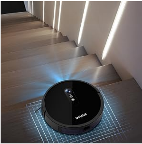
Anti-drop sensors detect edges and stairs, preventing the robot from falling.
