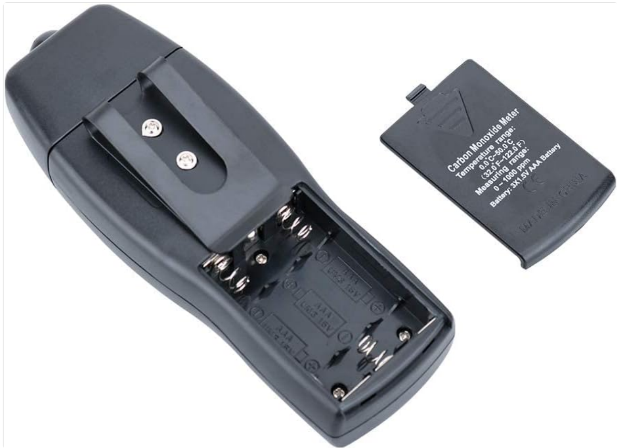
Image 5.1: Battery compartment for AAA batteries.
