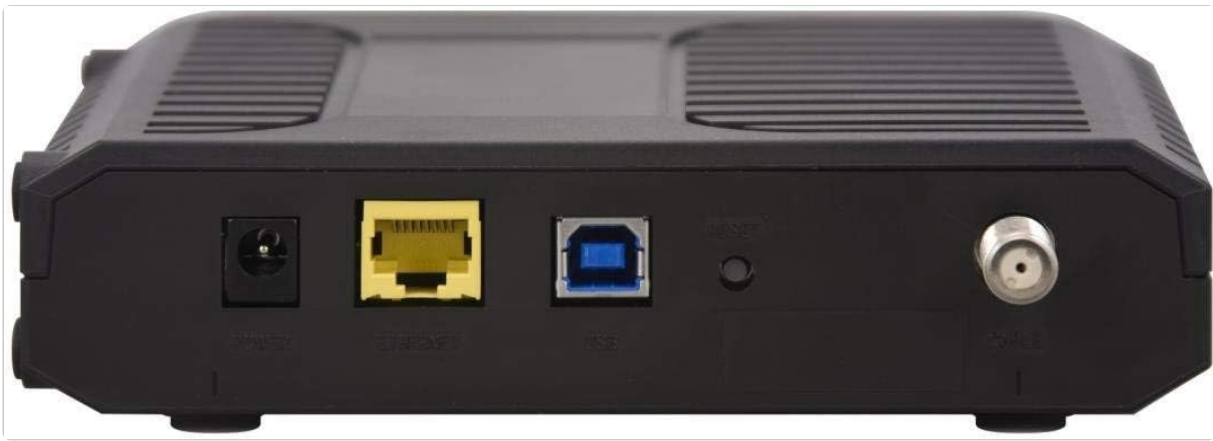
Figure 3: Rear view of the Cisco DPC3010 Cable Modem. This image displays the modem's rear ports, including the Power input, Ethernet port, USB port, Reset button, and Coaxial cable connector.
