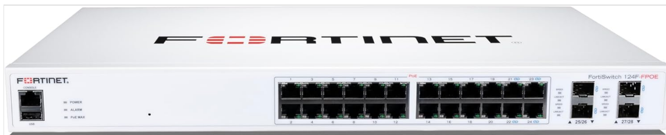
Figure 1: Front view of the Fortinet FortiSwitch 124F-POE, showing 24 PoE ports and uplink ports.
