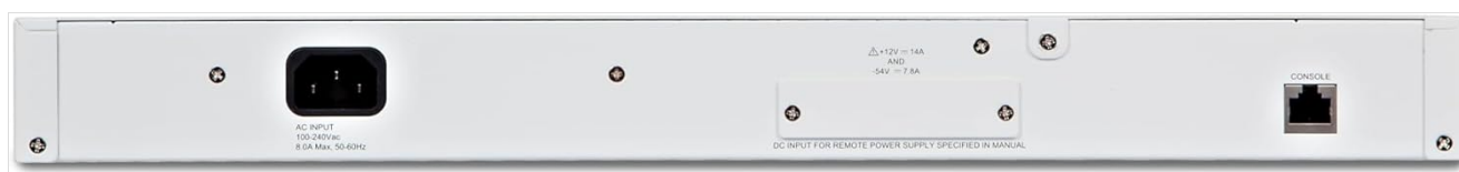
Figure 4: Rear view of the FortiSwitch 124F-POE, showing the AC input and console port.
