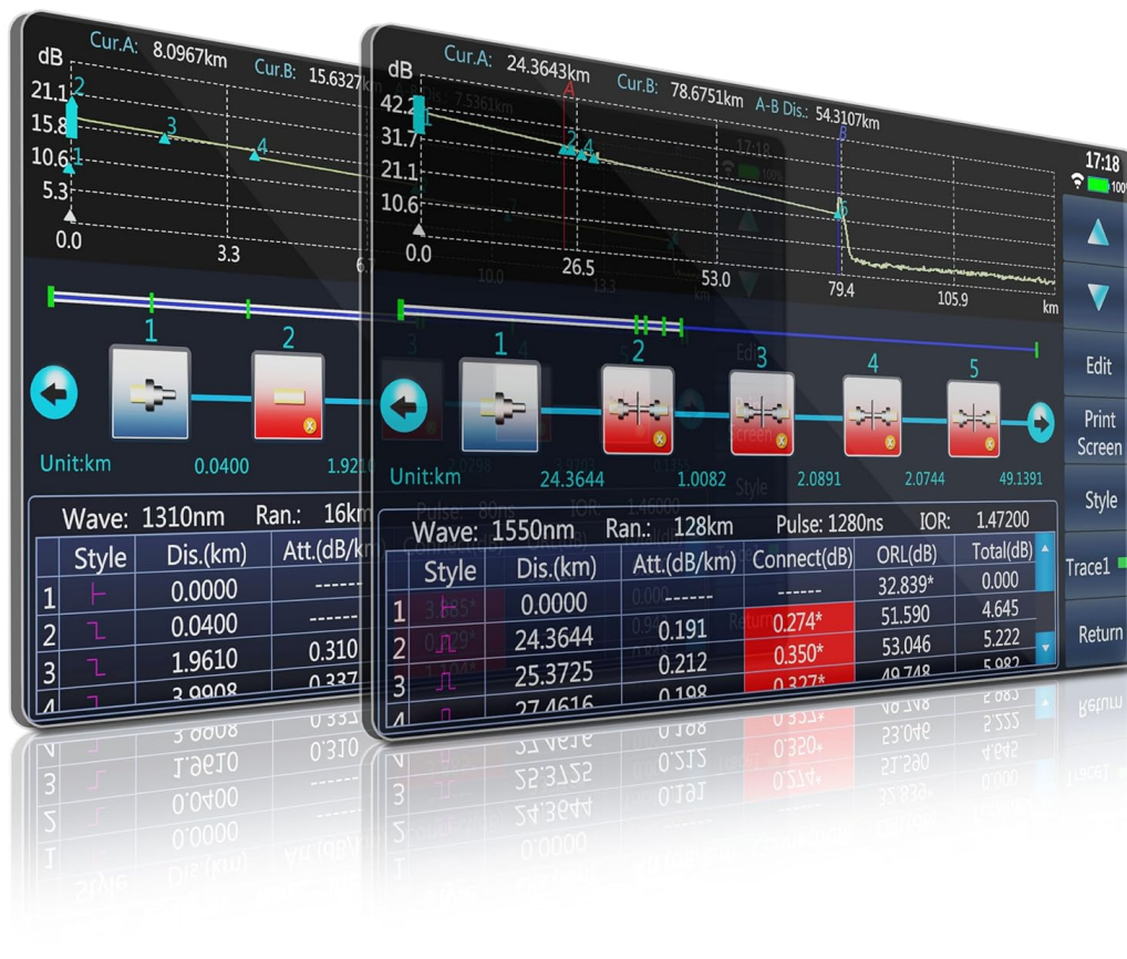
Figure 5: Example of 1310nm and 1550nm graphics analysis on the OTDR screen, detailing events and their characteristics.
