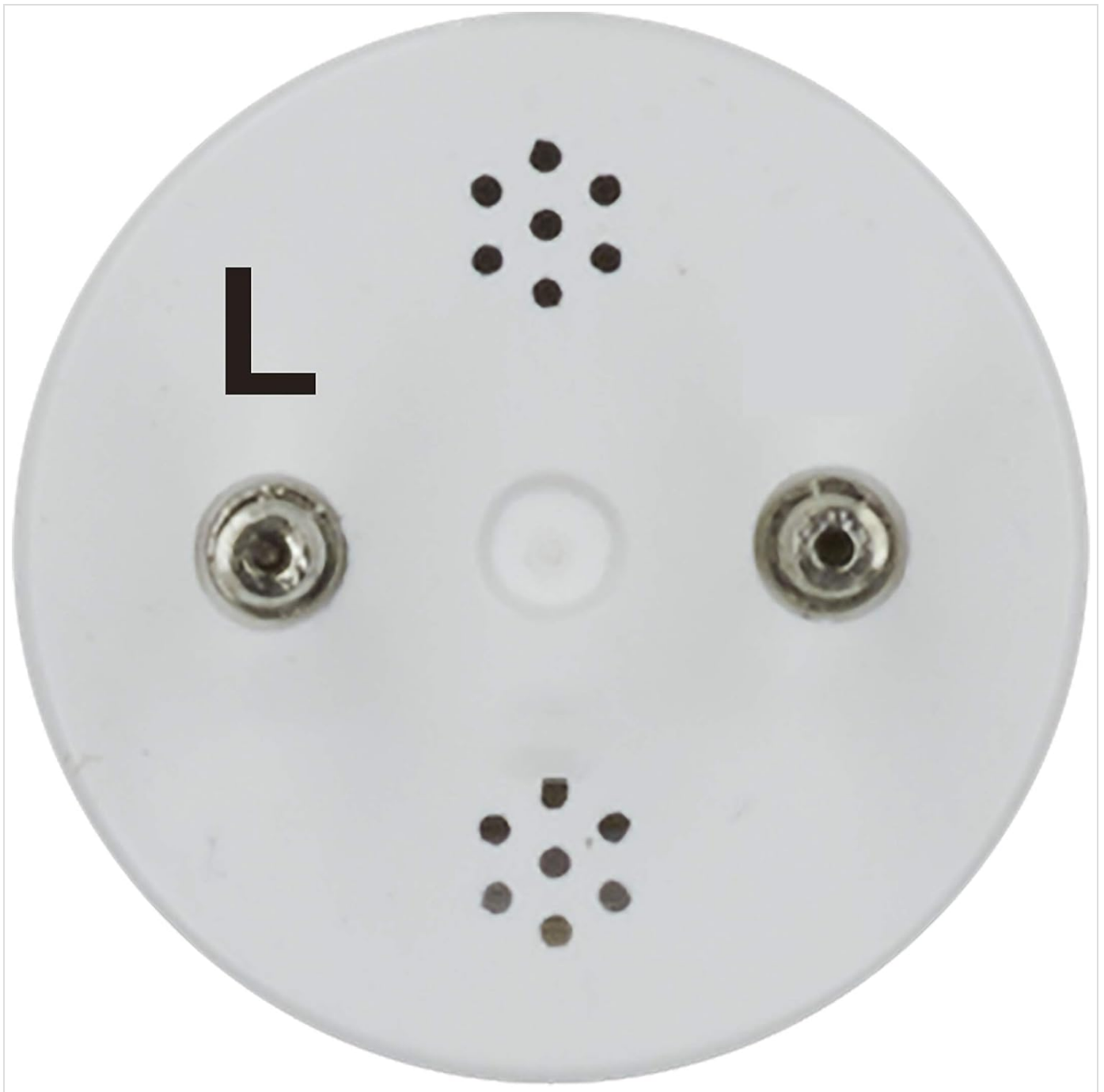
Image: Close-up of an LED tube end cap showing one pin labeled 'L' (Line), indicating where the Line power should be connected for double-ended wiring. The Neutral connection would be on the opposite end of the tube.
