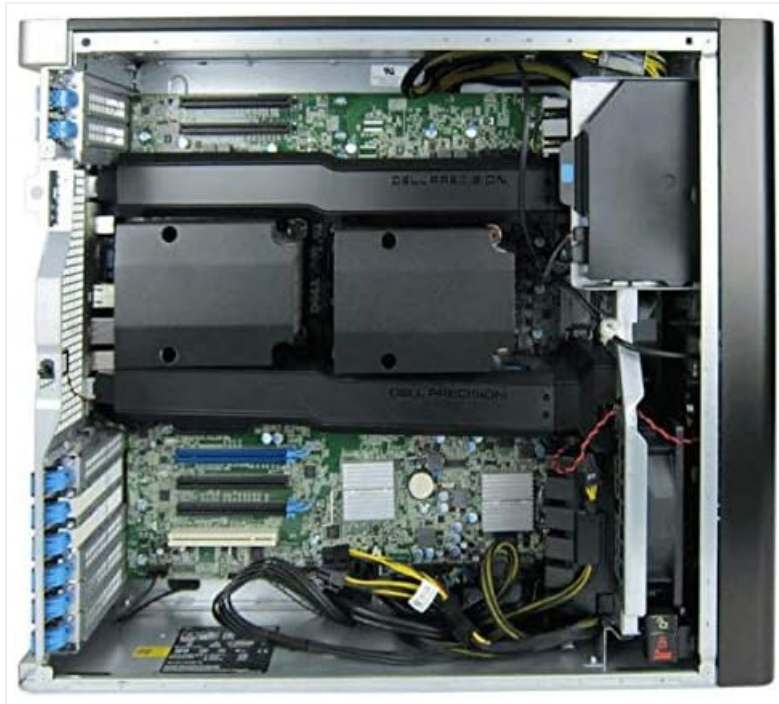
Figure 3: Internal view of the Dell Precision 7910 / T7910 Tower, highlighting the dual CPU heatsinks, RAM slots, and expansion card areas for maintenance and upgrades.
