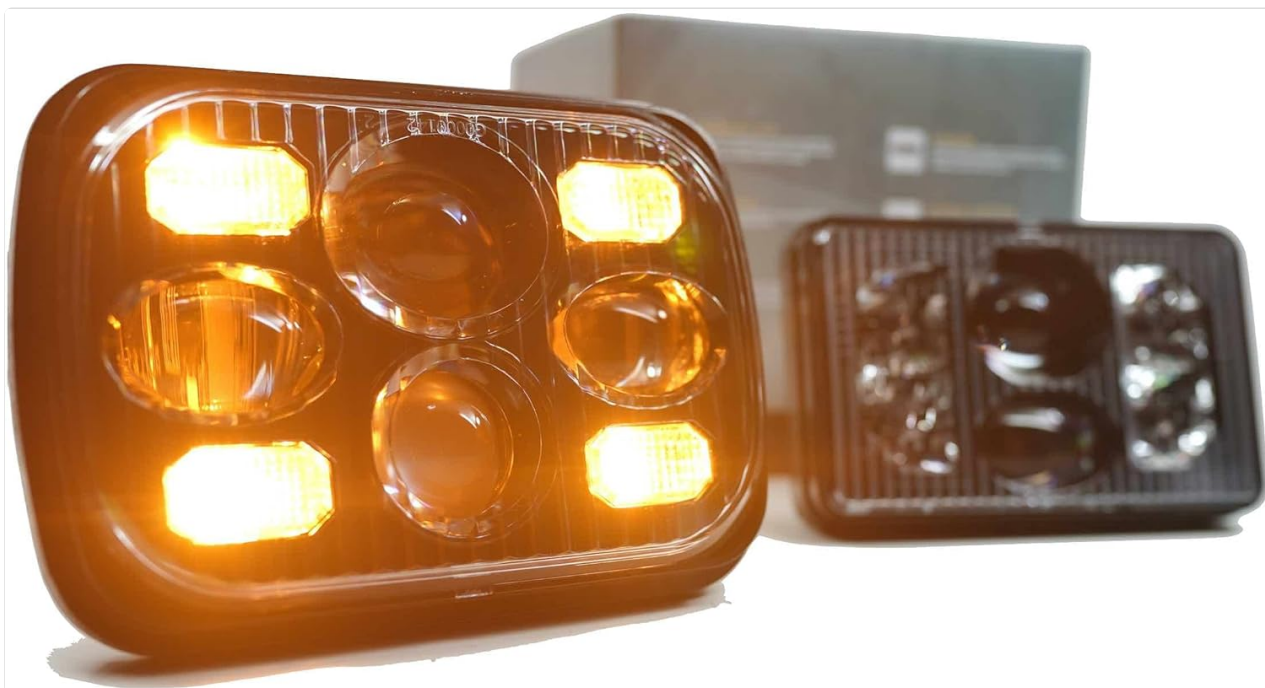
Figure 4.2: The Morimoto Sealed5 LED Headlights demonstrating the amber illumination of the switchback turn signal function.
