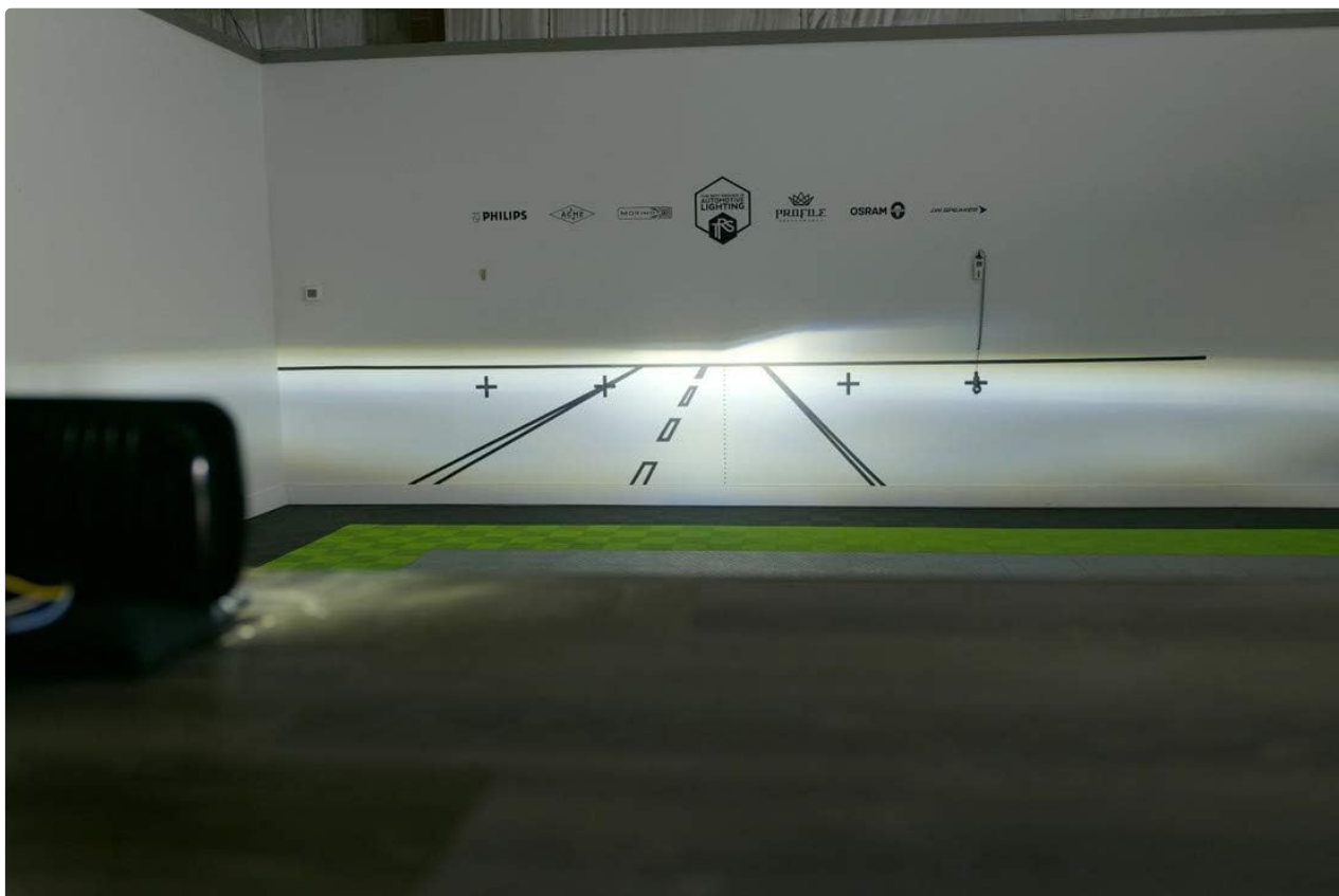
Figure 4.3: Example of the low beam pattern projected by the Morimoto Sealed5 LED Headlight, showing a clear cutoff line.
