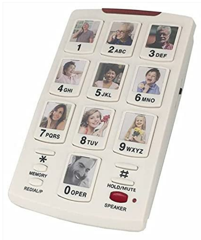
Figure 2.1: Front view of the ATS BBPhotoPhone, showcasing the large, customizable photo memory buttons and main control keys.
