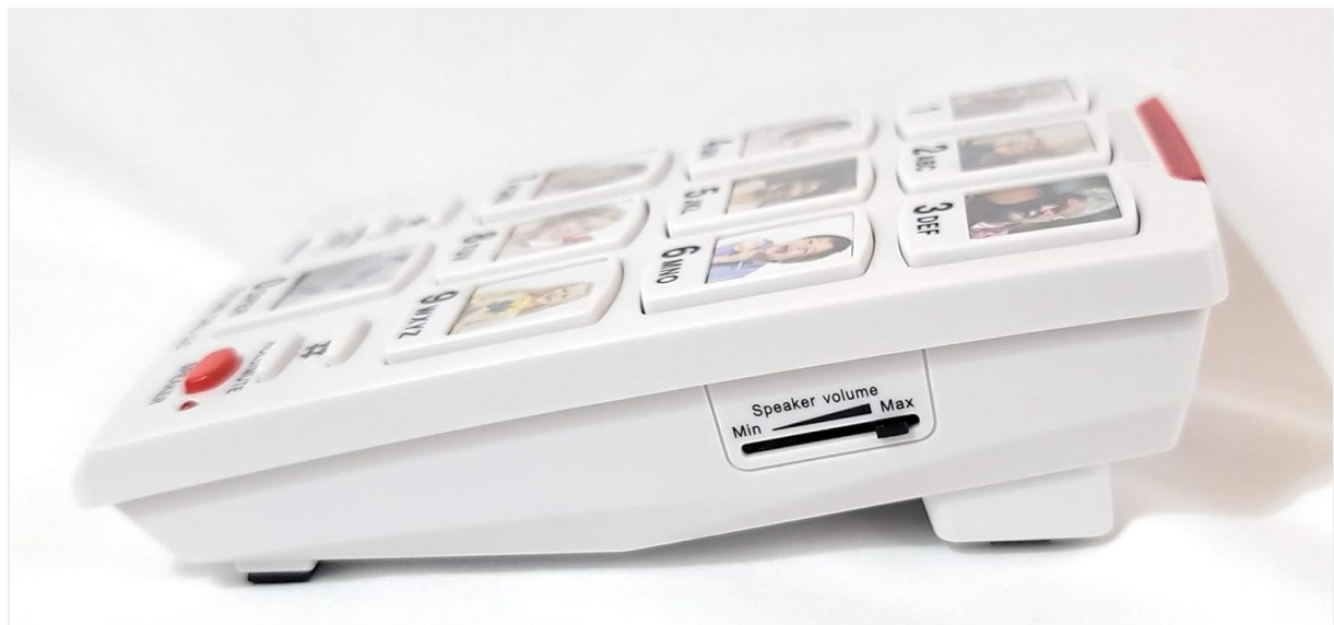
Figure 4.1: Side view of the BBPhotoPhone, indicating the location of the speaker volume slide control.
