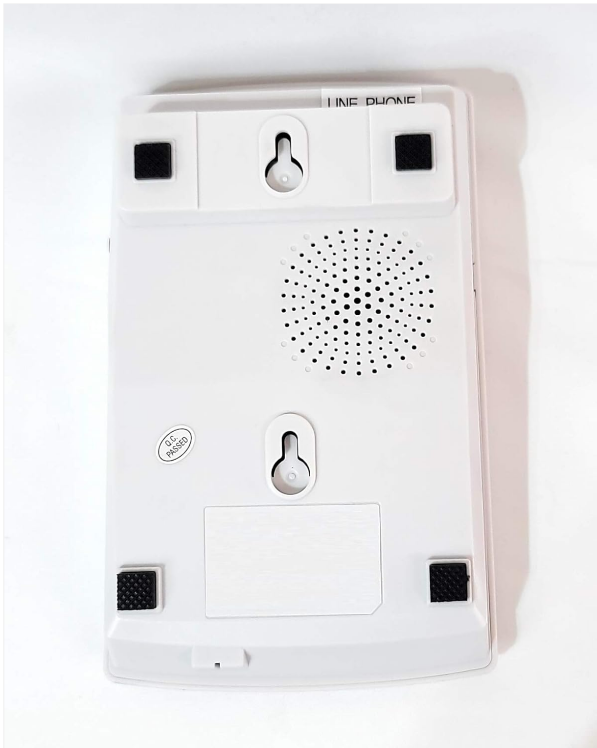
Figure 3.2: Bottom view of the BBPhotoPhone, highlighting the wall mounting slots and speaker grille.
