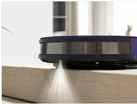
Figure 10: The anti-drop sensor on the robot vacuum, preventing falls from elevated surfaces.
