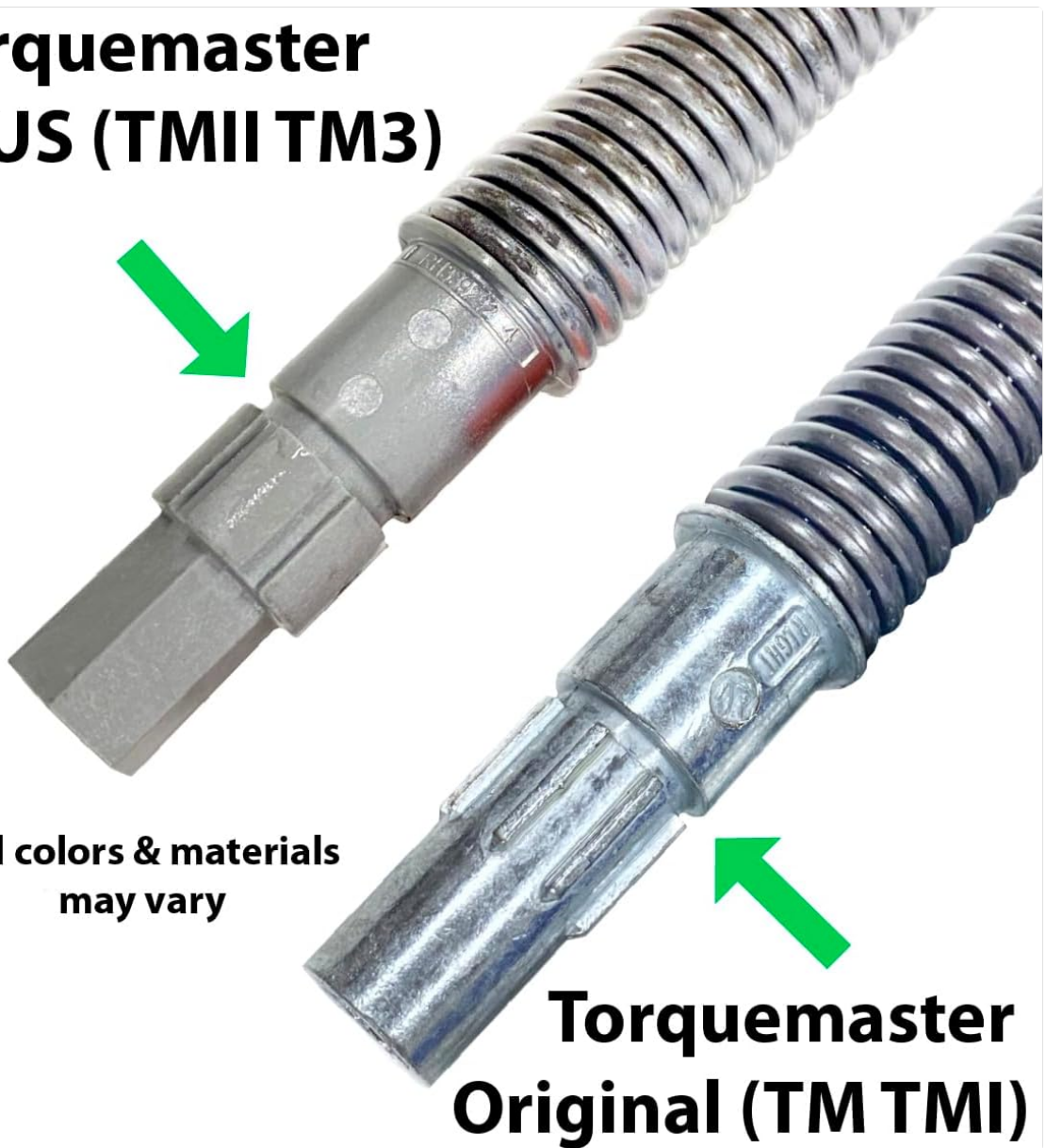
Image 1: Comparison of Torquemaster Plus (TMII TM3) and Torquemaster Original (TM TMI) spring winding ends. Note the hexagonal shape on the Torquemaster Plus end (top) versus the rounder, splined end of the Torquemaster Original (bottom).
