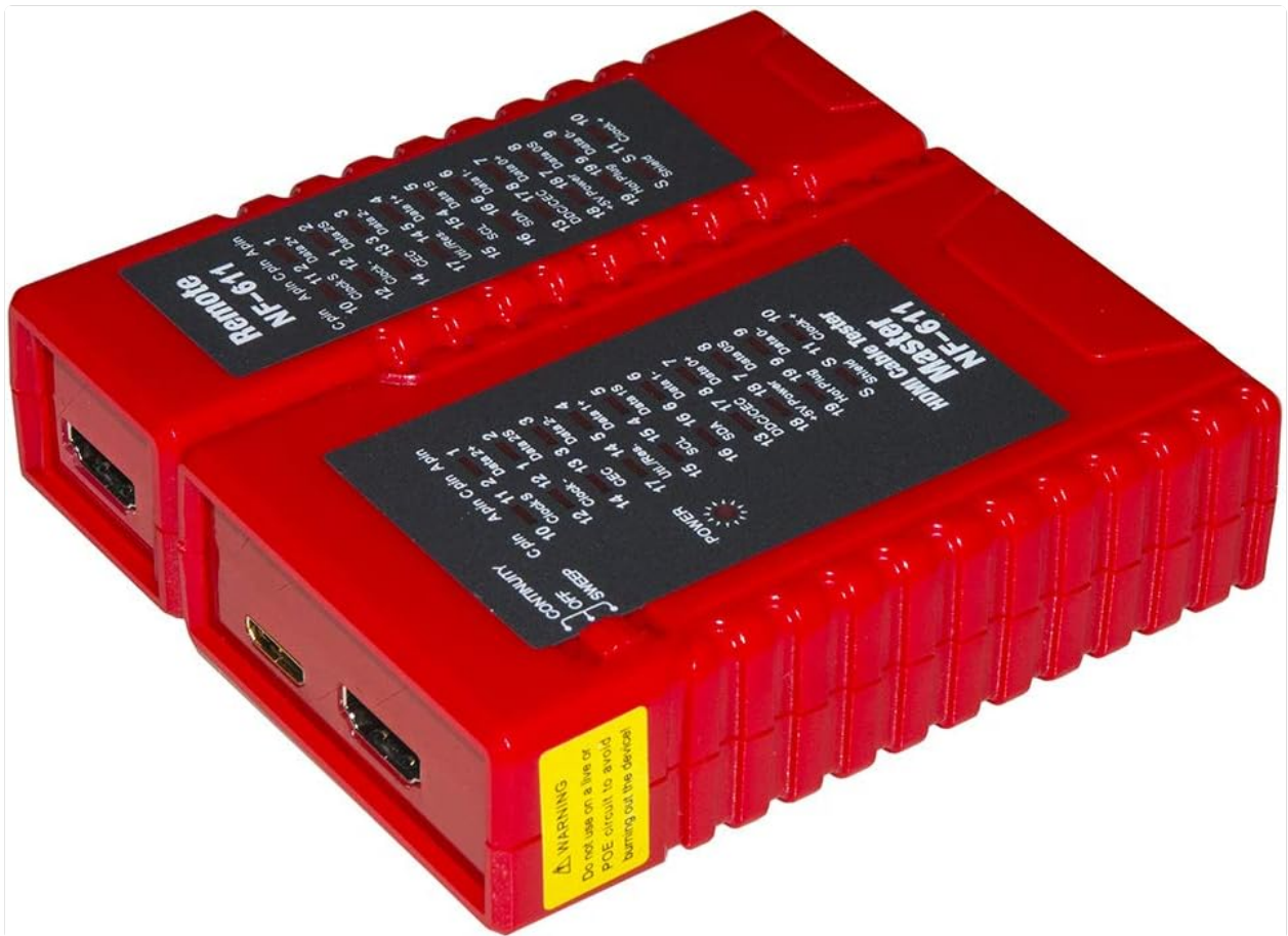
Image 2: The LINK LKMS06 HDMI Cable Tester with the Master and Remote units separated. This view highlights the HDMI Type A and Type C ports on each unit, which are used for connecting the HDMI cable under test. The separation allows for testing of longer cables where the remote end is distant from the master unit.
