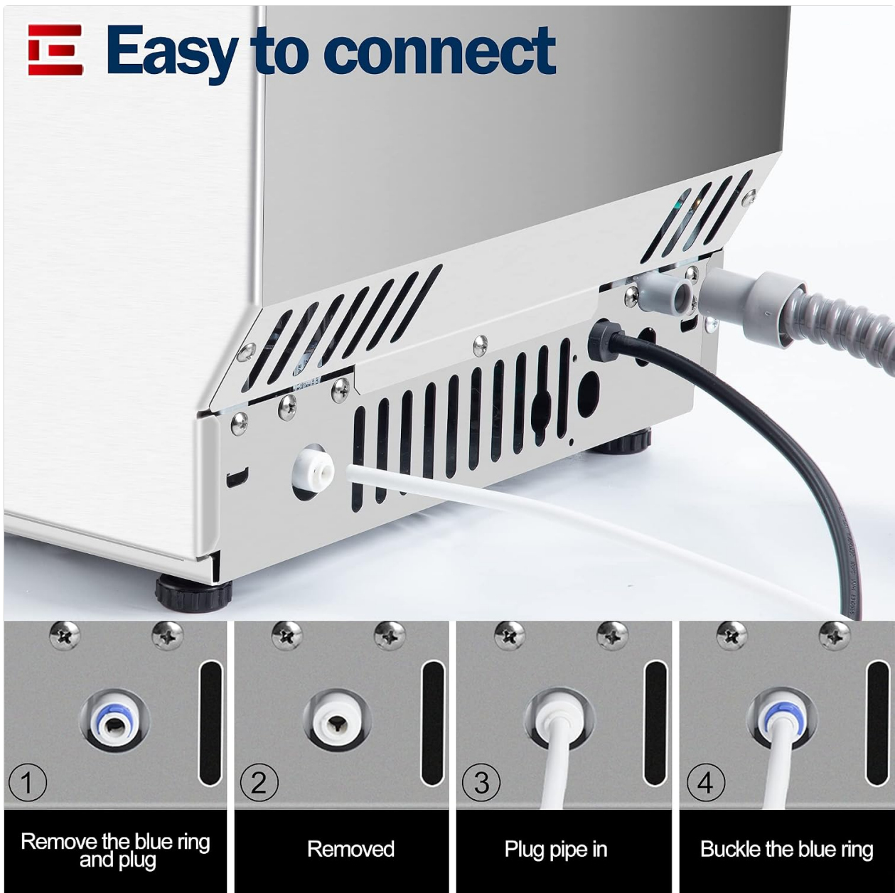
Figure 3.2: Detailed steps for connecting the water inlet pipe. This involves removing a plug, inserting the pipe, and securing it with a blue ring.
