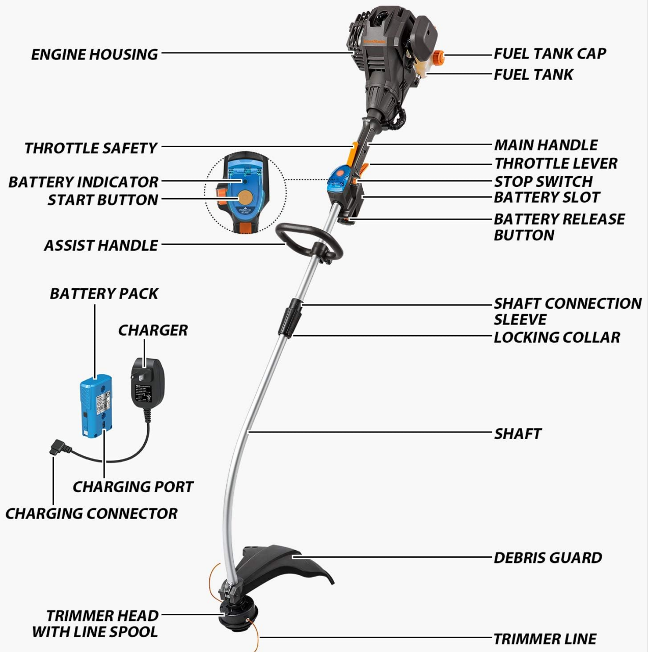
Figure 2.1: Exploded view of the LawnMaster NPTGCP2517B string trimmer, highlighting key components such as the engine housing, fuel tank, main handle, throttle lever, electric start button, battery slot, shaft, debris guard, and trimmer head.
