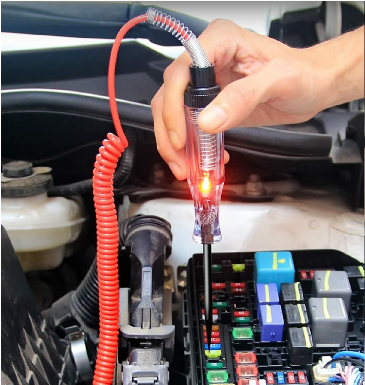
Figure 6.1: Using the circuit tester to check fuses in a vehicle's fuse box.
