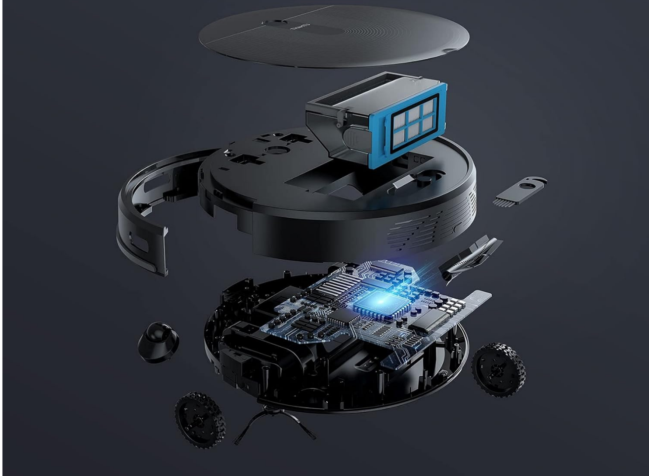
Figure 1: Exploded view of the Thamtu G11 Robot Vacuum Cleaner, showing its internal components such as the dustbin, main brush, side brushes, and wheels.
