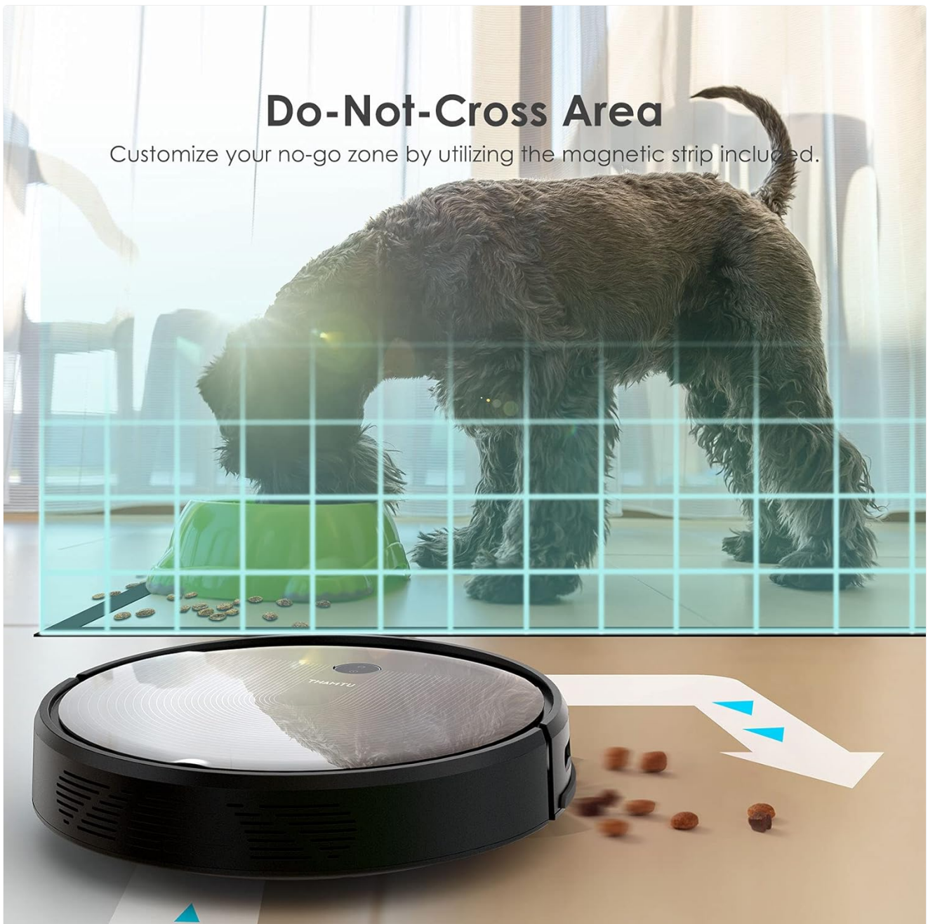
Figure 3: The Thanttu G11 robot vacuum respects magnetic boundary strips, preventing it from entering designated "no-go" zones, such as around pet food bowls.
