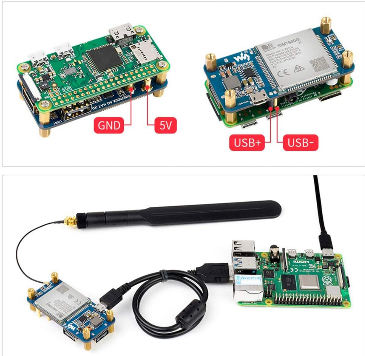
Figure 2: Connection of the SIM7600G-H module to a Raspberry Pi Zero using pogo pins.
