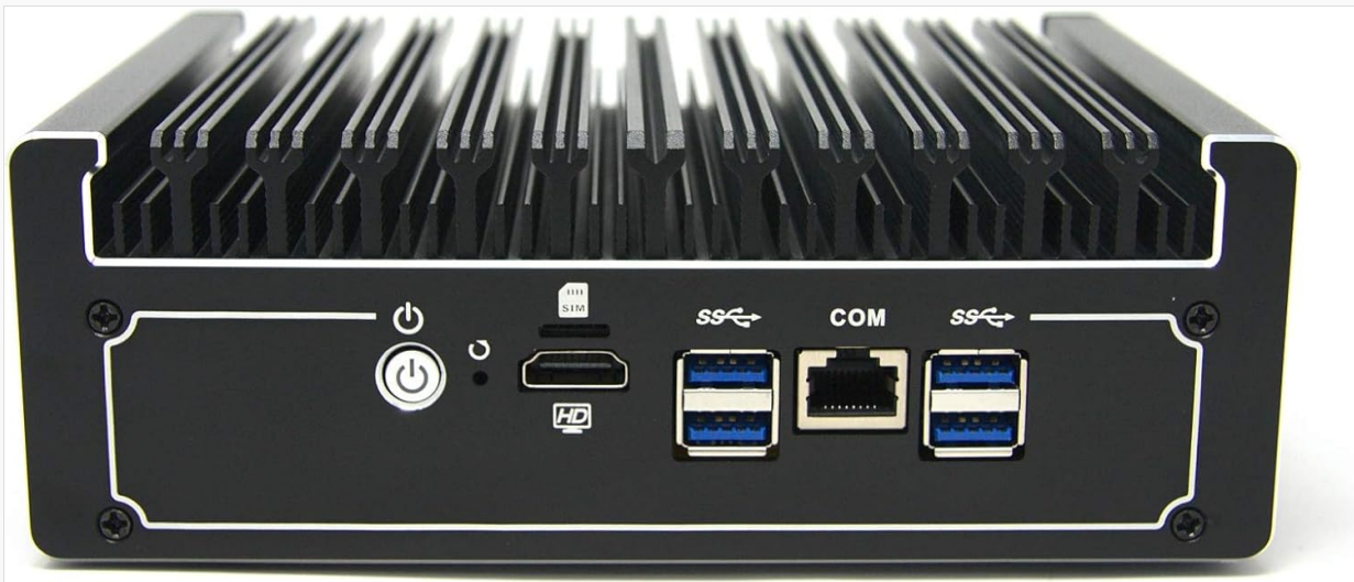
Image: Front panel of the Protectli Vault, including the power button, four USB 3.0 ports, an HDMI port, and a COM port.
