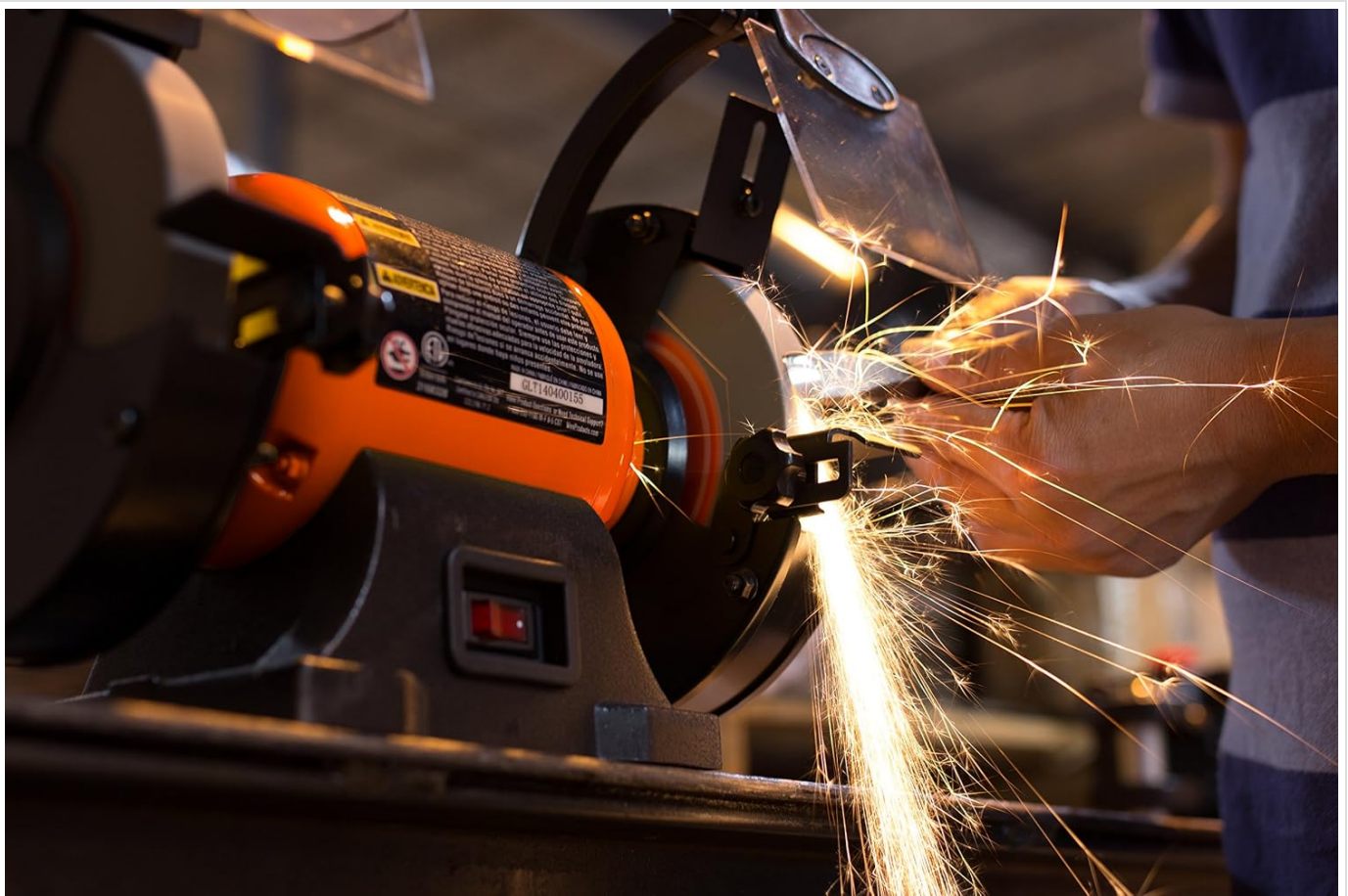
Image 5.1: A user operating the WEN BG4276 Bench Grinder, demonstrating the process of grinding a metal object, with sparks visible, emphasizing the importance of eye protection.
