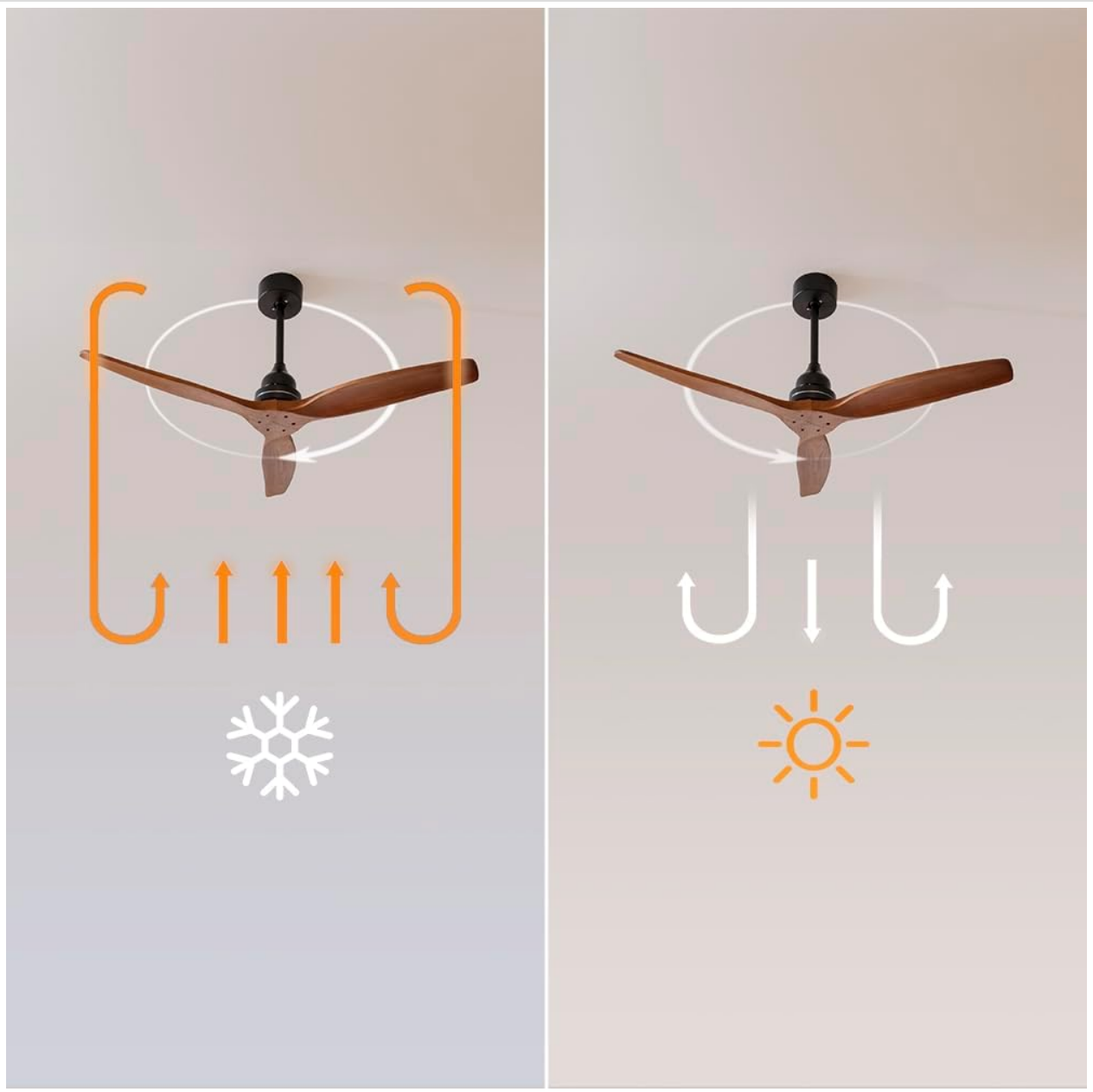
Image: A visual diagram explaining how the fan's rotation direction changes airflow for cooling in summer and heat distribution in winter.
