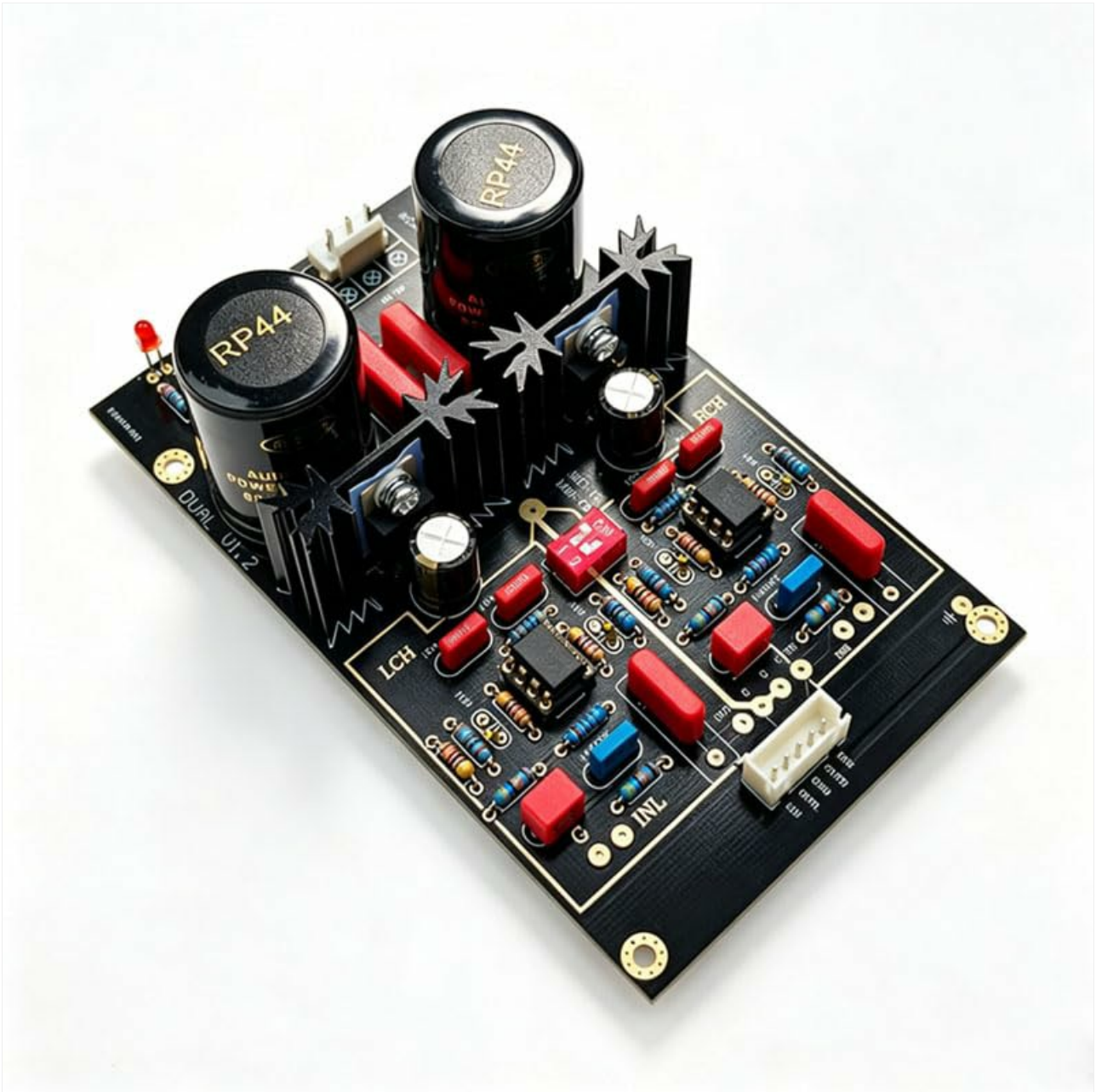
Figure 1: Top-down view of the Reland Sun DUAL Phono Preamplifier board. This image shows the layout of the capacitors, resistors, operational amplifiers (LME49720NA/NE5532), and input/output terminals.
