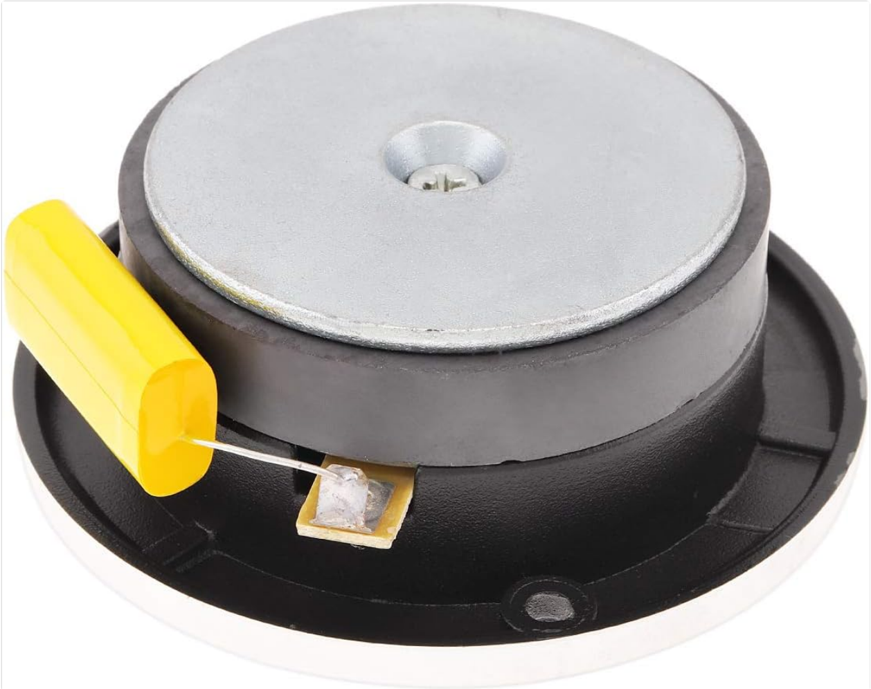
Figure 5.1: Side profile of the tweeter, highlighting the yellow capacitor connected to the wiring terminal.
