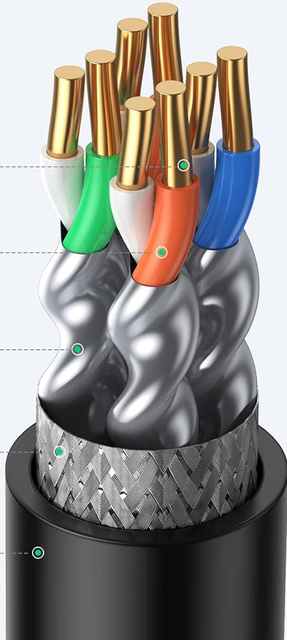
Figure 6: Cross-section diagram of the S/FTP Double Shielding of the Cat 8 cable, detailing 26AWG Copper Core, Twisted Pair Wires, Aluminum Foil, Metal Mesh, and PVC Jacket.
