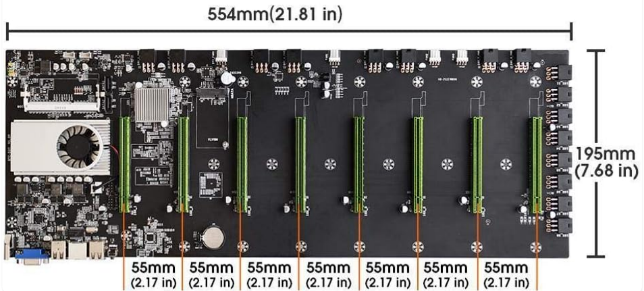
Figure 2: Overview of the BTC-D37 motherboard's key features and physical dimensions.
