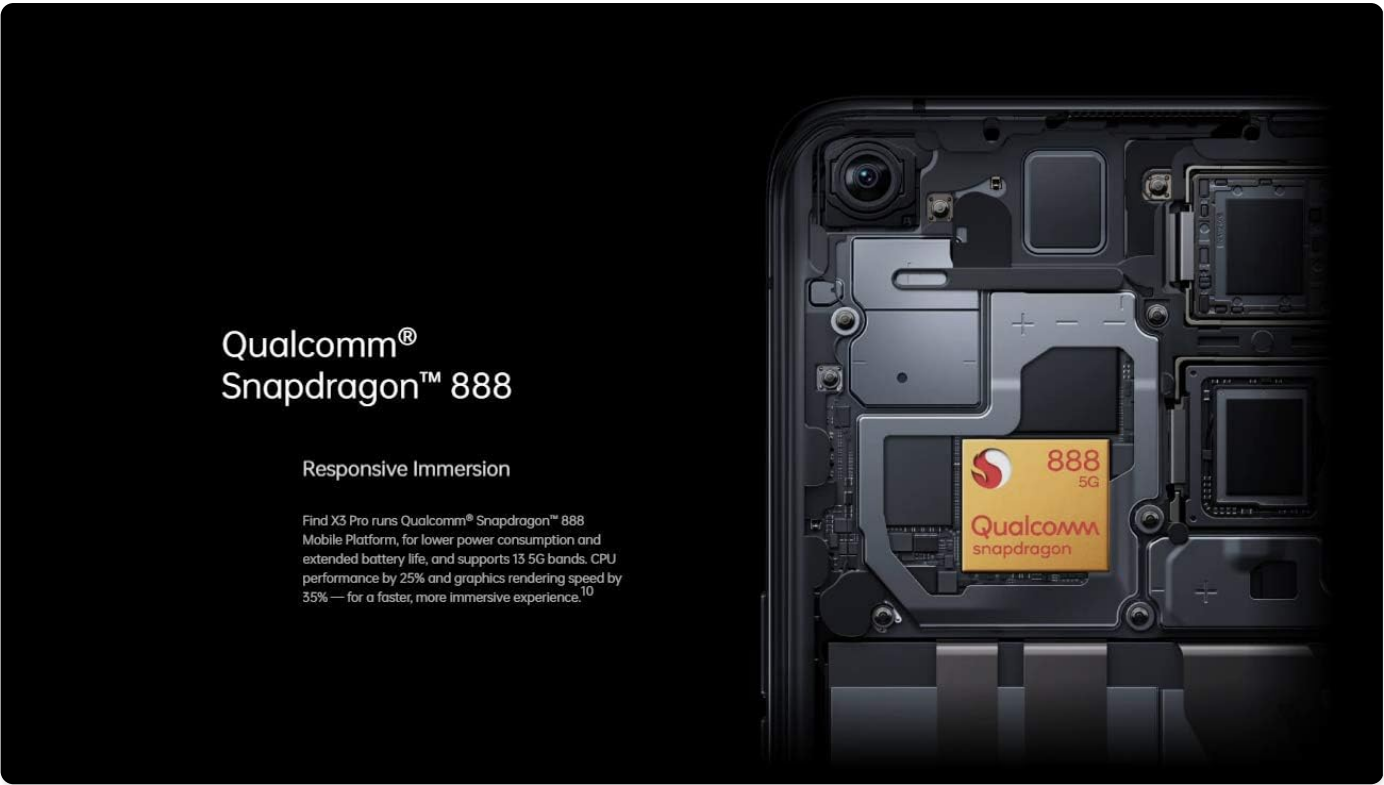
Image 3.3: Internal view highlighting the Qualcomm Snapdragon 888 Mobile Platform, responsible for the phone's high performance and 5G capabilities.
