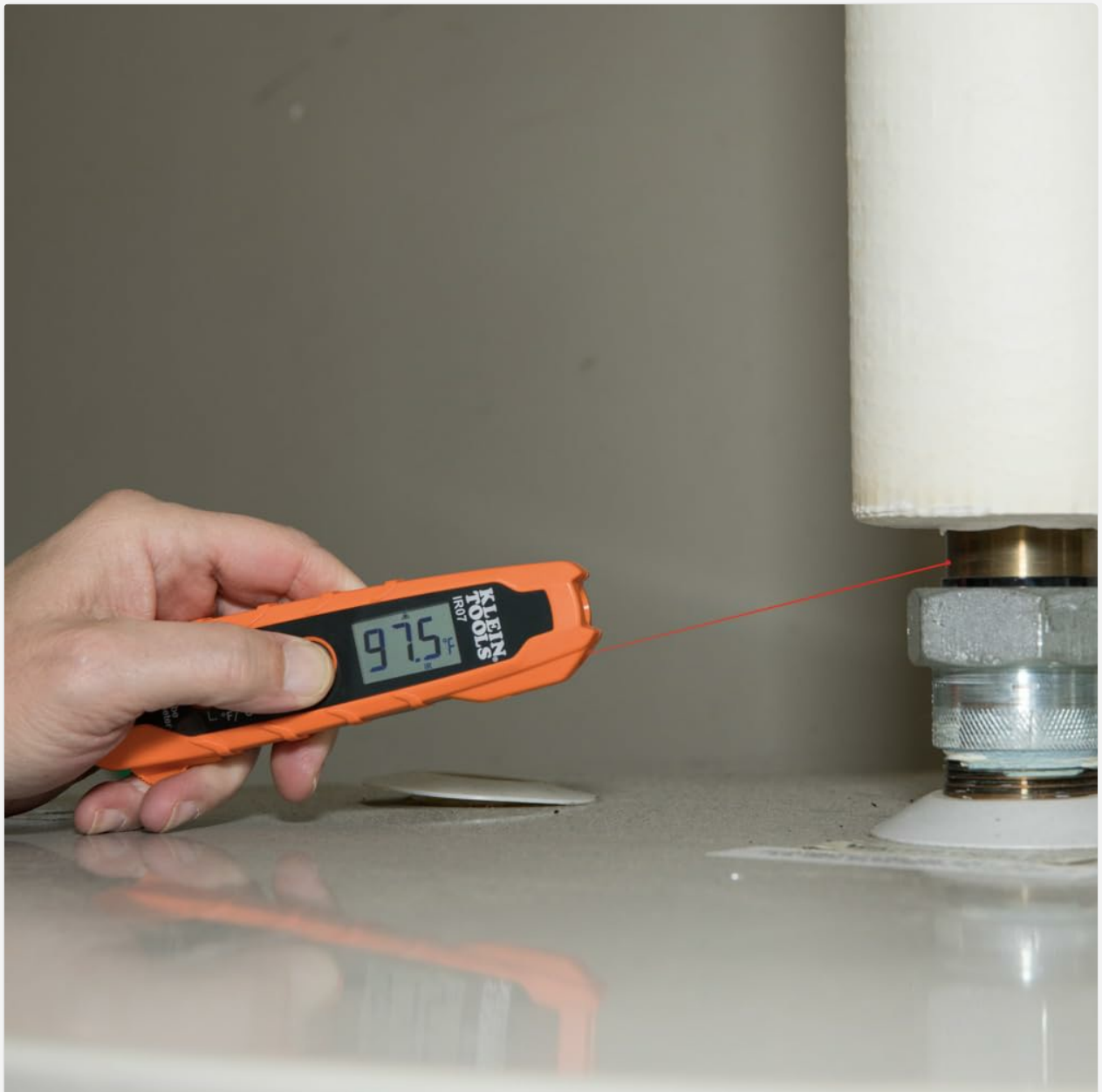
Figure 6: Measuring surface temperature with the IR07 Thermometer.
