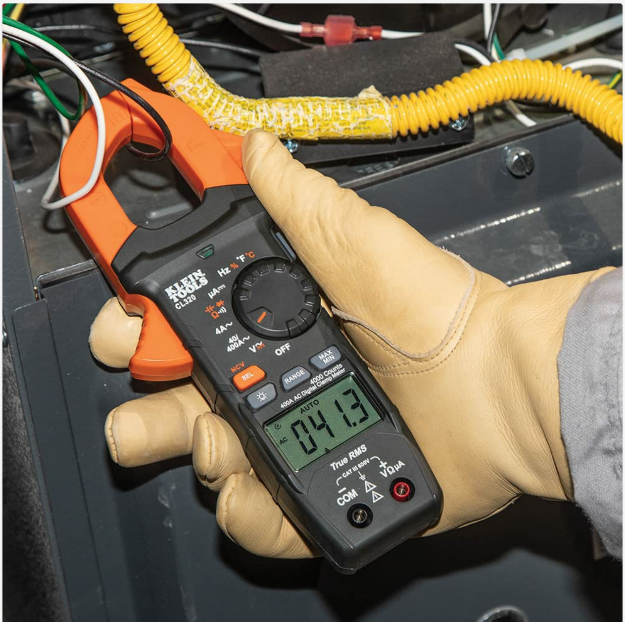
Figure 5: Measuring AC current with the CL320 Clamp Meter.
