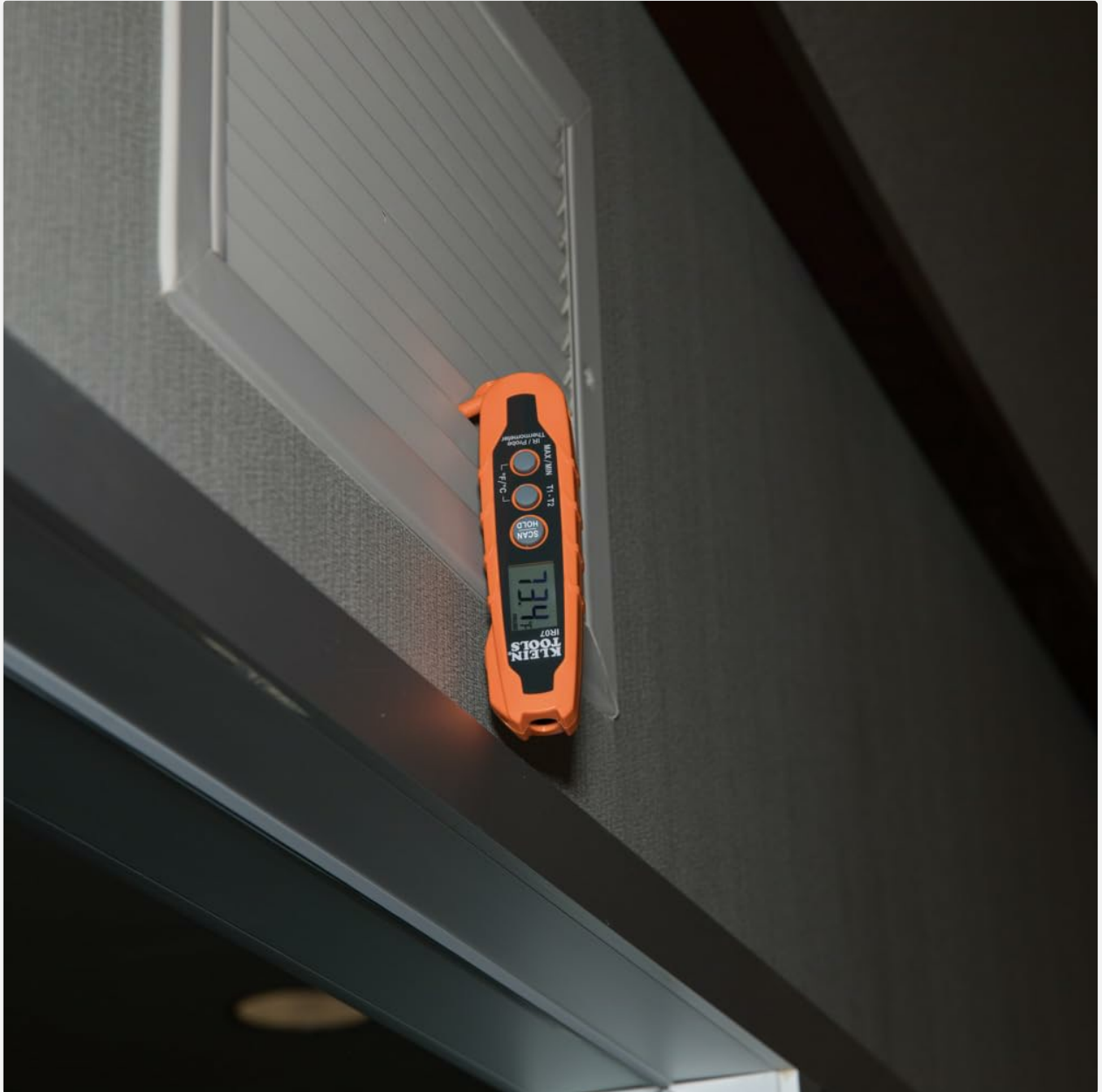
Figure 7: Measuring air temperature with the IR07 Thermometer probe.
