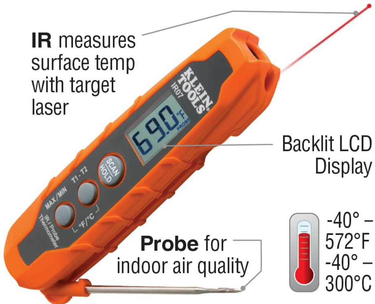
Figure 3: Key features of the IR07 Dual IR and Probe Thermometer.
