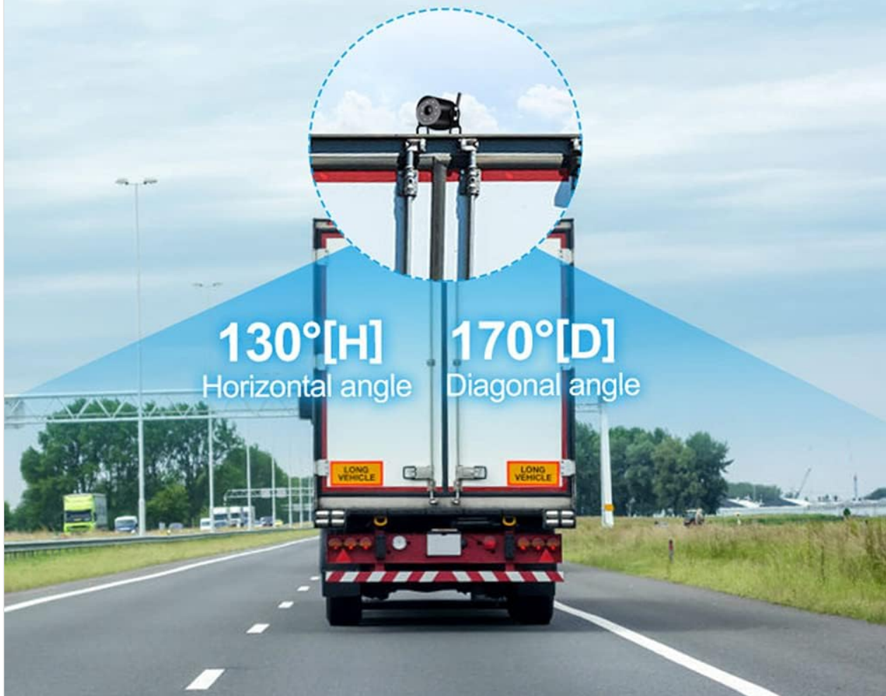
Figure 5.3: Camera's wide view angle (130° Horizontal, 170° Diagonal).
