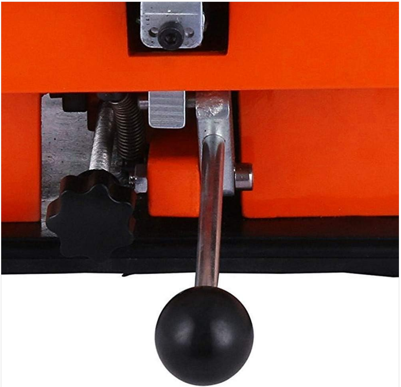
Figure 6: The stamping lever, which is used to apply pressure for embossing characters.
