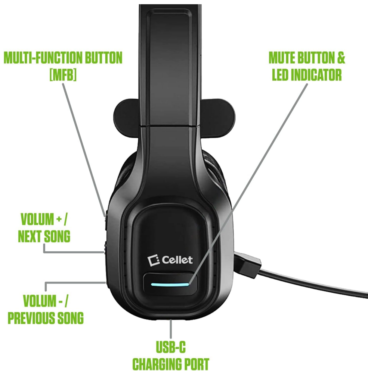
Image: Diagram illustrating the multi-function button (MFB), volume up/next song, volume down/previous song, mute button & LED indicator, and USB-C charging port on the headset.
