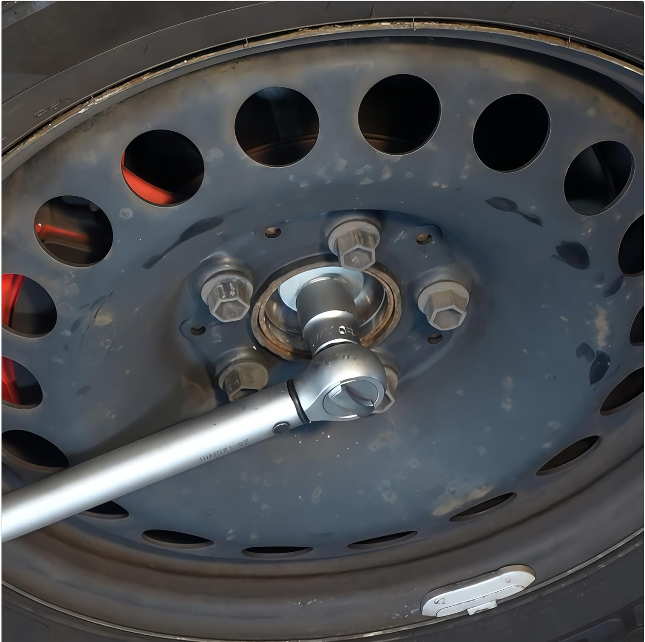
Image 4.1: Using a socket with a torque wrench.
