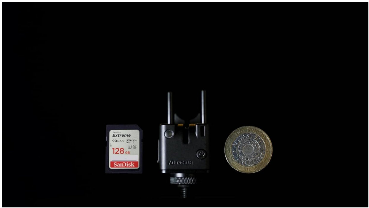
Image 2.2.2: An N1 bite alarm shown next to an SD card and a coin for size comparison, illustrating its compact design.
