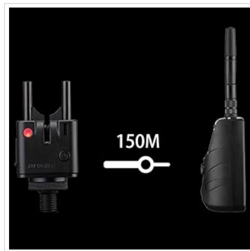
Image 4.4.1: An N1 bite alarm and the S9r receiver depicted with a "150M" indicator, signifying the maximum operational range.
