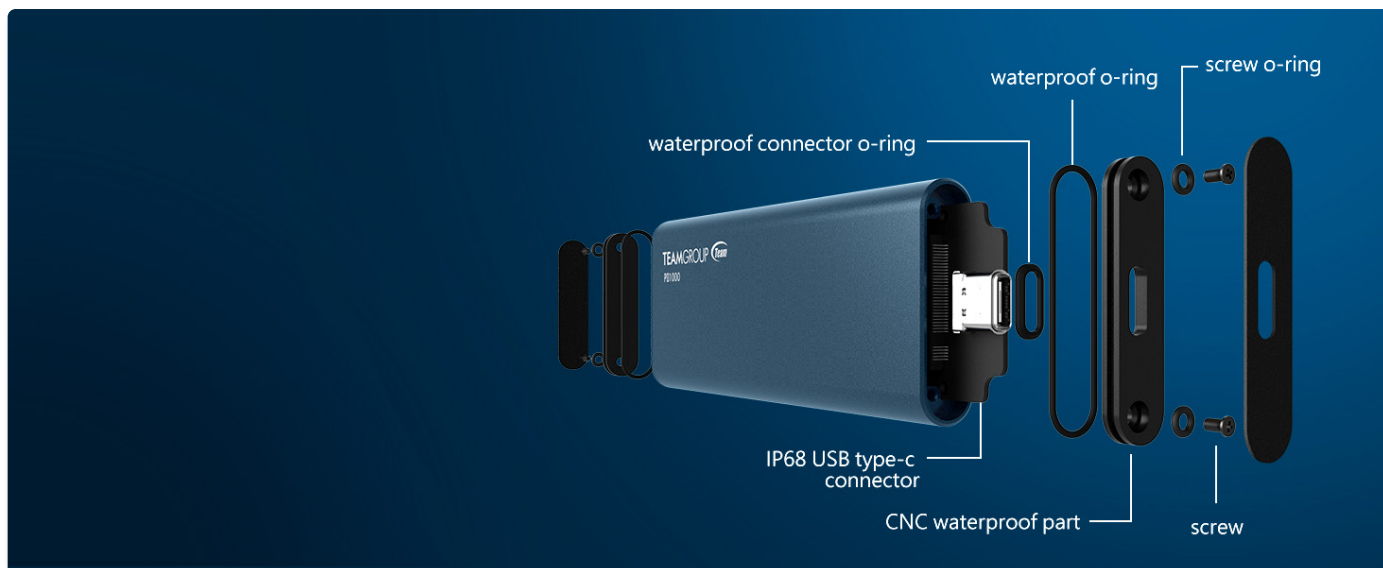
An exploded diagram of the TEAMGROUP PD1000 SSD, detailing its internal components and the waterproof sealing mechanisms, including O-rings and the IP68 USB Type-C connector.
